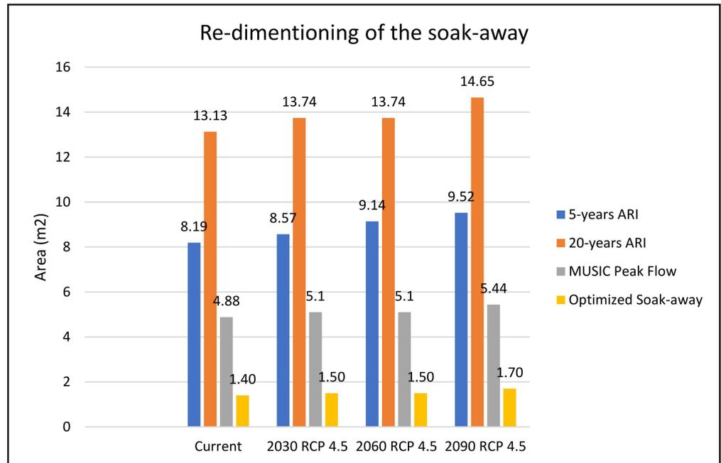
Figure 4. Re-dimensioning of the soak-away for RCP 4.5.
