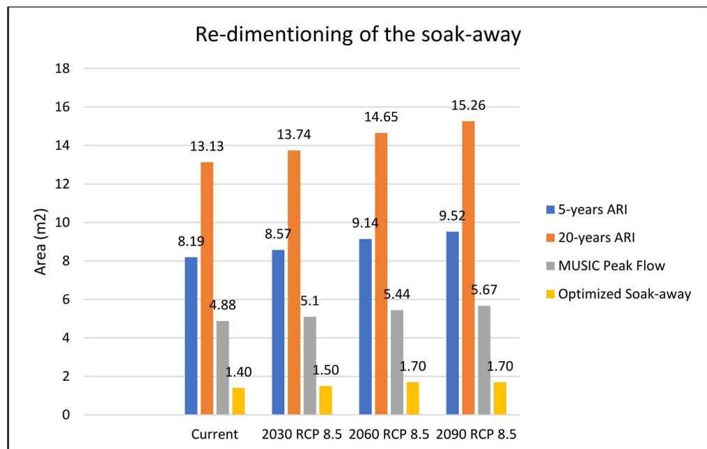
Figure 5. Re-dimensioning of the soak-away for RCP 8.5.
