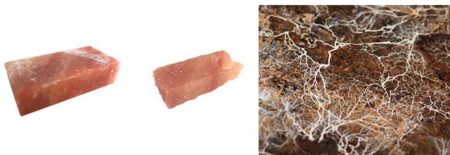
**Figure 2.** The salt brick and Mogud mycelium brick.
