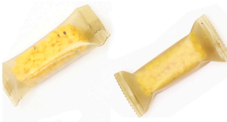
**Figure 18.** Different contents of beeswax in two biofilms. **Left:** Beeswax is 5 g, which accounts for 2.25% of the overall solution (sample S4.1); **Right:** Beeswax is 15 g, which accounts for 6.75% of the overall solution (S4.3).
