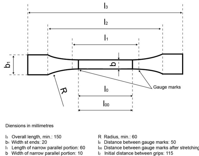
Figure 10. Strength test specific values.
