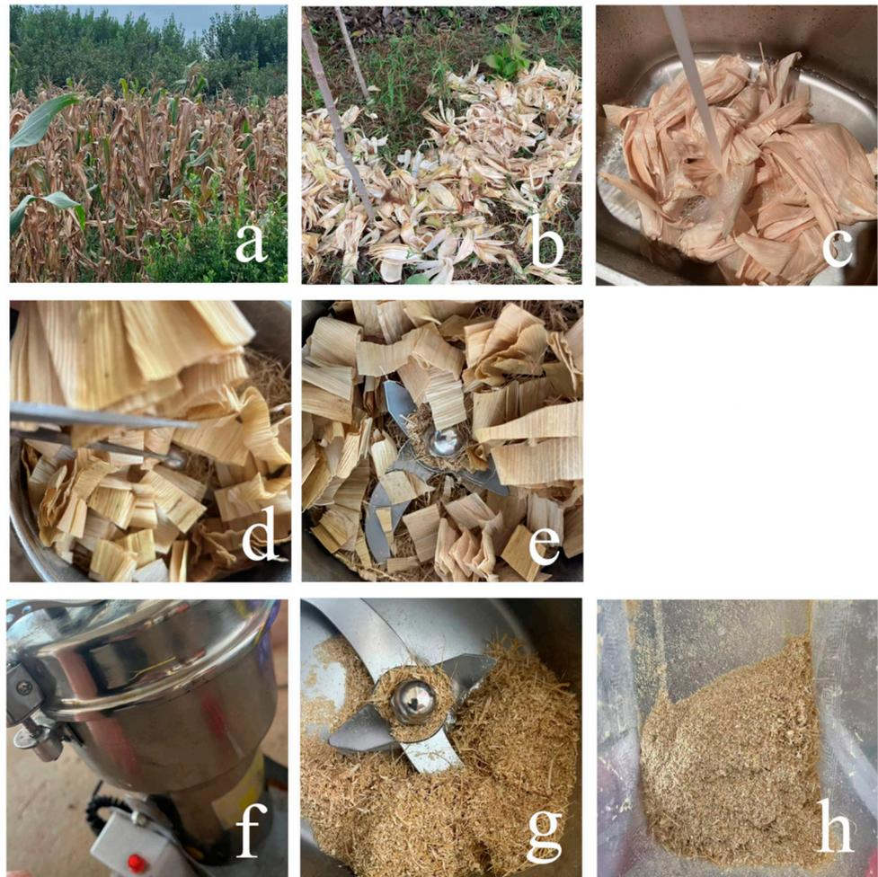
**Figure 4.** The handling process of corn stover: (a) corn stalks in original state, (b) initial material collection, (c) filtering and cleaning, (d–h) grinding process.
