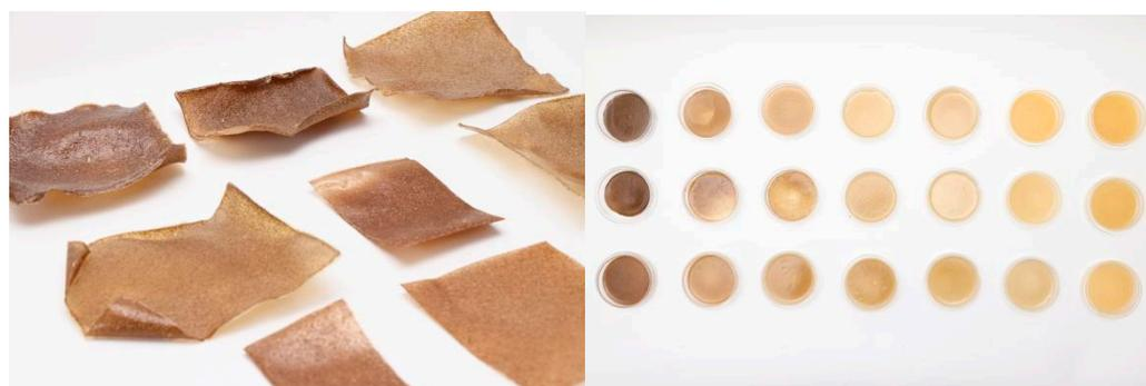
**Figure 6.** Partial samples: the two images display different effects achieved by adding powder of varying concentrations (the colour from dark to light represents the quantity of corn waste powder added from a high to low concentration); **Left** image: the original shapes of films with different corn waste powder concentrations; **Right** image: a comparative view of the films after processing (trimming).
