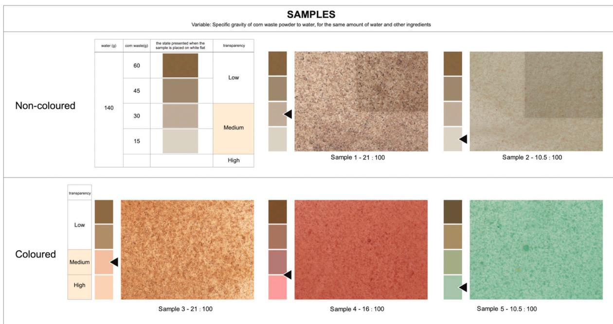
**Figure 13.** Comparing test samples to analyse transparency and colourability: first row: transparency experiment, second row: coloured experiment.
