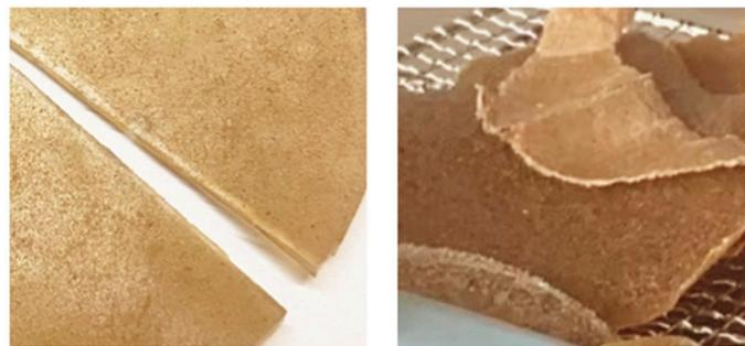
**Figure 15.** Left: S2.1 biomaterial fracture due to external forces; Right: S3.1 fragments and powder at the fracture point.
