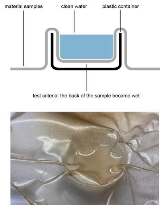
**Figure 12.** Above: Schematic of waterproof test; Below: Real picture of waterproof test.
