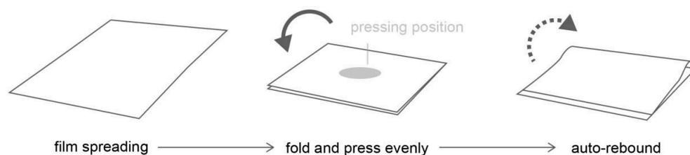
**Figure 9.** Three steps of the elasticity test method; the line and arrow in the upper left corner of the middle picture represents the direction when fold and press, and the dotted arrow in the right picture represents the path of the material's automatic rebound.
