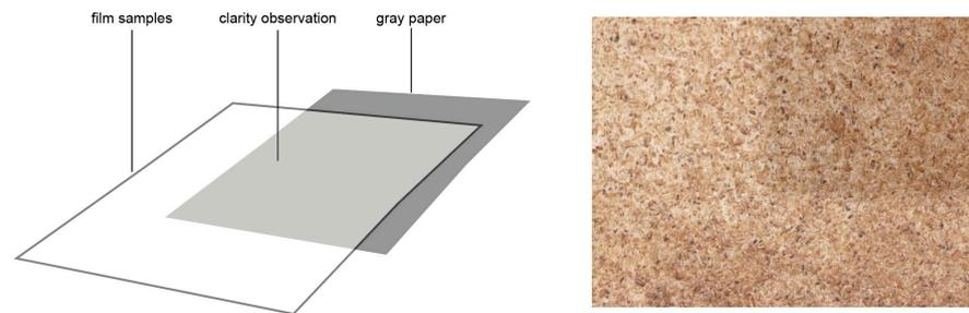
**Figure 7.** The grey paper was covered under a film to observe the visual state (**left:** sketch map; **right:** real effect).
