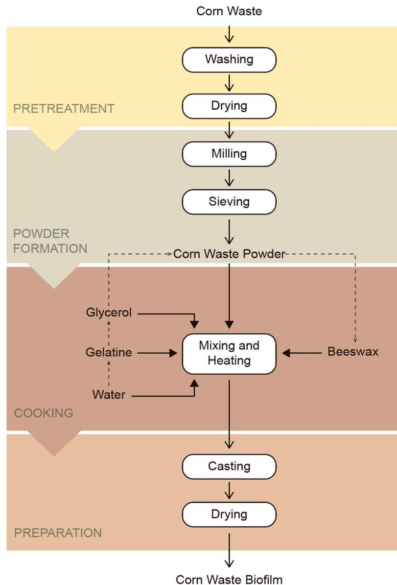
**Figure 3.** The processing flow chart; dotted lines with arrows indicate the order in which ingredients are added.
