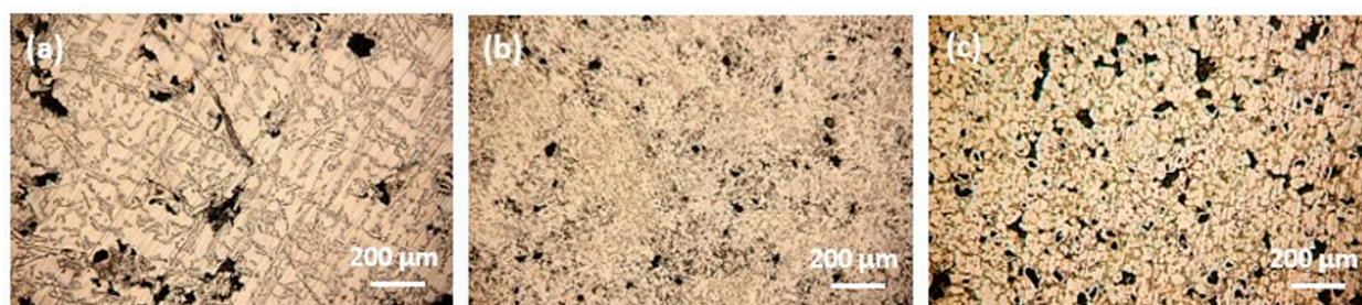
Figure 8. Optical microscopy images of the electrode surfaces after PD measurements in NaCl: (a) RS, (b) DHES, and (c) TFS.
