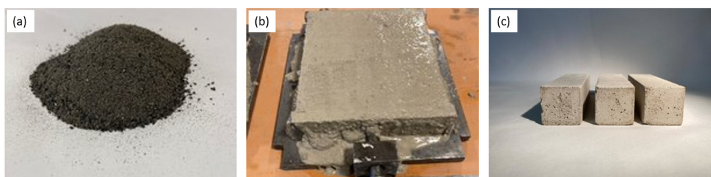
Figure 6. Production of OW_A mortars: (a) OW_A ; (b) molding phase; (c) prismatic specimens after demolding and curing.
