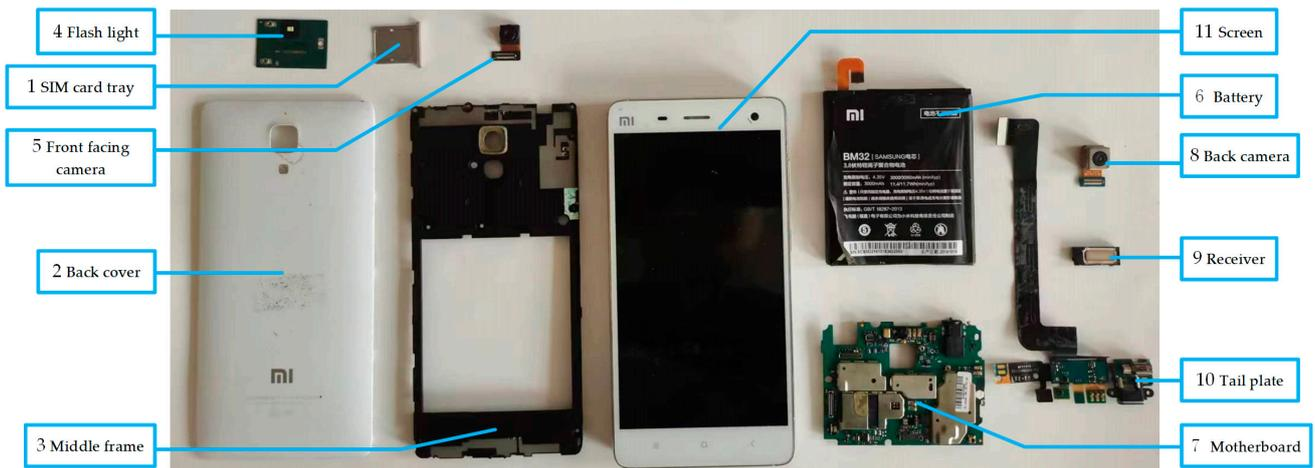
Figure 7. The disassembly parts graph for 'Xiaomi 4'.
