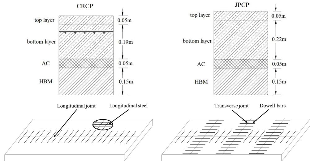
**Figure 3.** Layer structure and top view of CRCP and JPCP in the test section; AC: asphalt concrete interlayer; HBM: hydraulically bound material.
