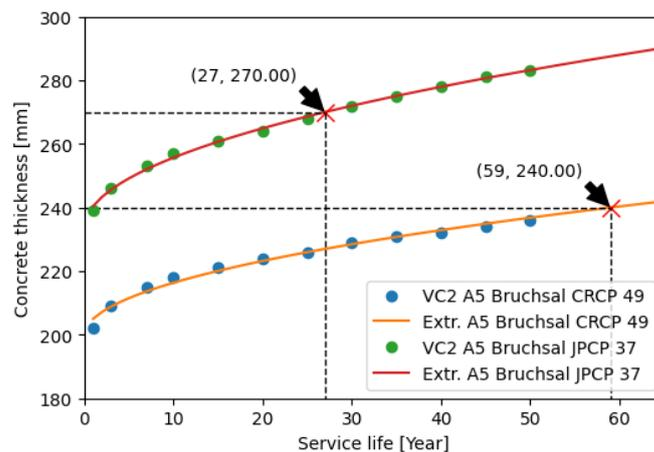
**Figure 4.** Calculation of the service life of the examined construction methods in VENCON 2.0.
