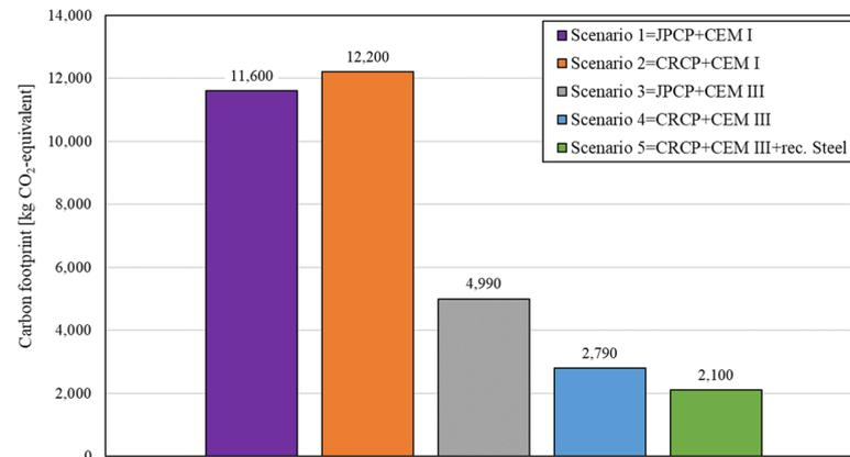
Figure 12. Carbon footprint of the CRCP and JPCP.
