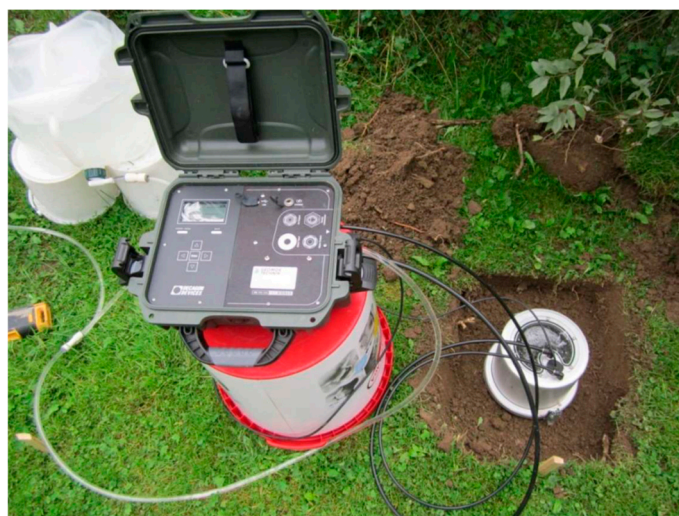
Figure 5. View of the research station for testing the infiltration coefficient with the Saturo infiltrometer (photo by M. Cholewa).
