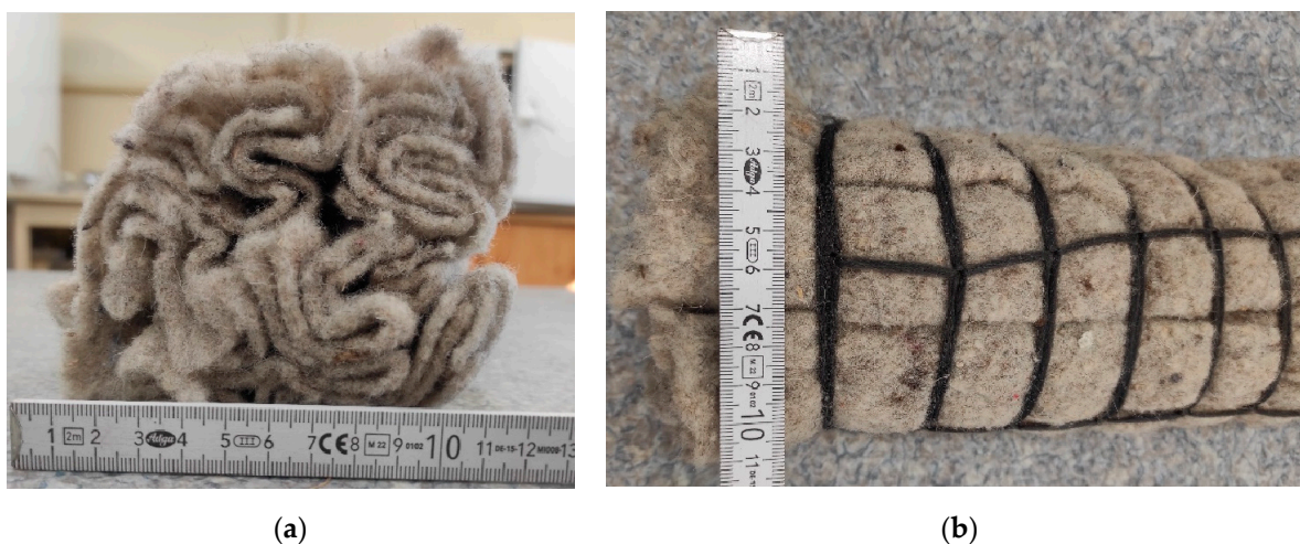
Figure 7. View of the 100 mm diameter Kemafil georope used in the study (photo by A. Gruchot): (a) cross section of Kemafil georope; (b) top view of the Kemafil georope, visible a string braid.
