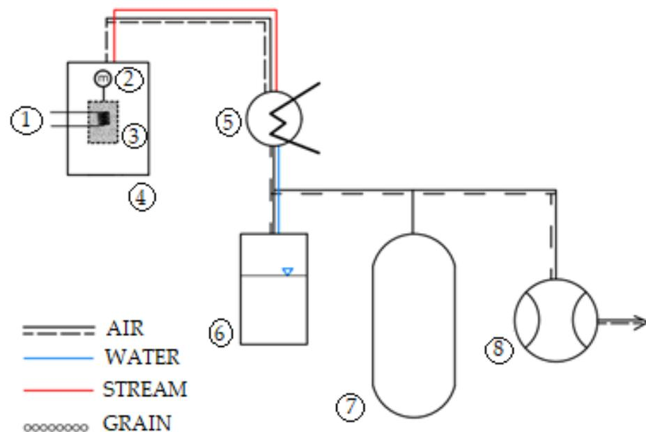
**Figure 1.** Diagram of the simplified physical model of a vacuum dryer [38], where 1—electric heating, 2—tensometric balance, 3—perforated basket for the grain, 4—vacuum chamber, 5—condenser, 6—condensate tank, 7—vacuum air reservoir and 8—vacuum pump.
