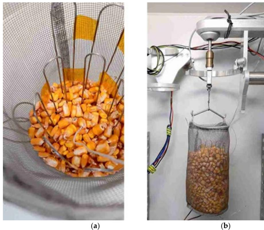
**Figure 2.** Perforated grain basket and electric heating coils for grain heating [38]: (a) detail and (b) scale for determining the weight of the grain sample, along with the basket and the heating coils.
