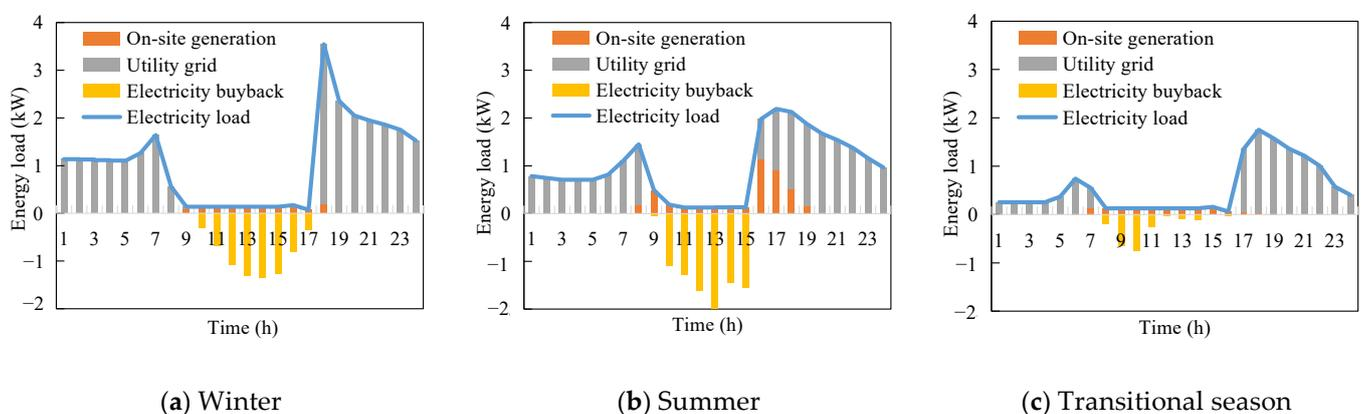
**Figure 4.** Electrical balance of the PV system on typical days.
