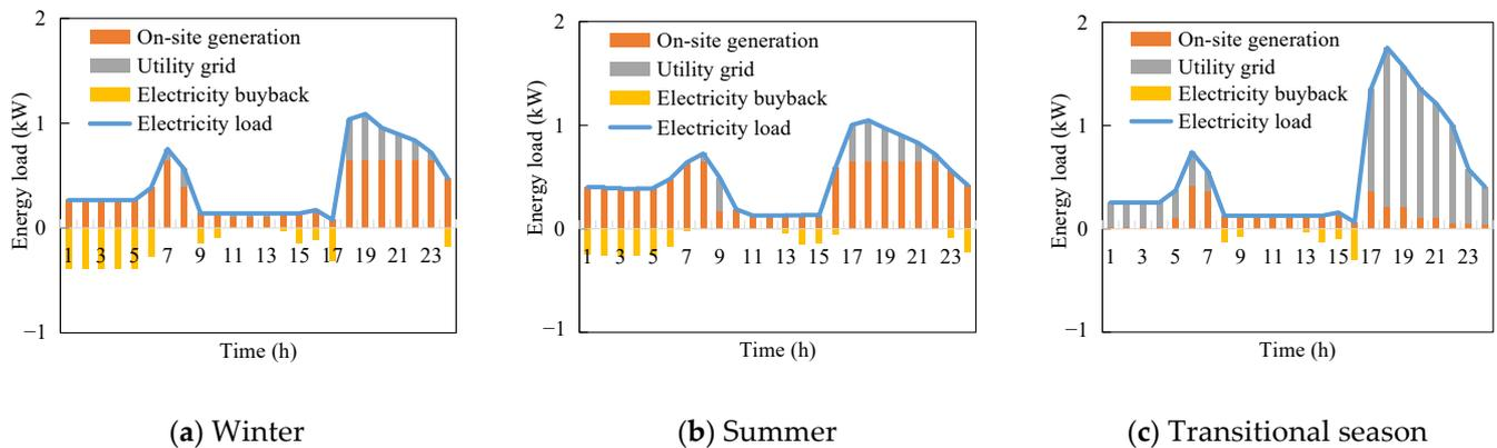
Figure 5. Electrical balance of the CCHP system on typical days.
