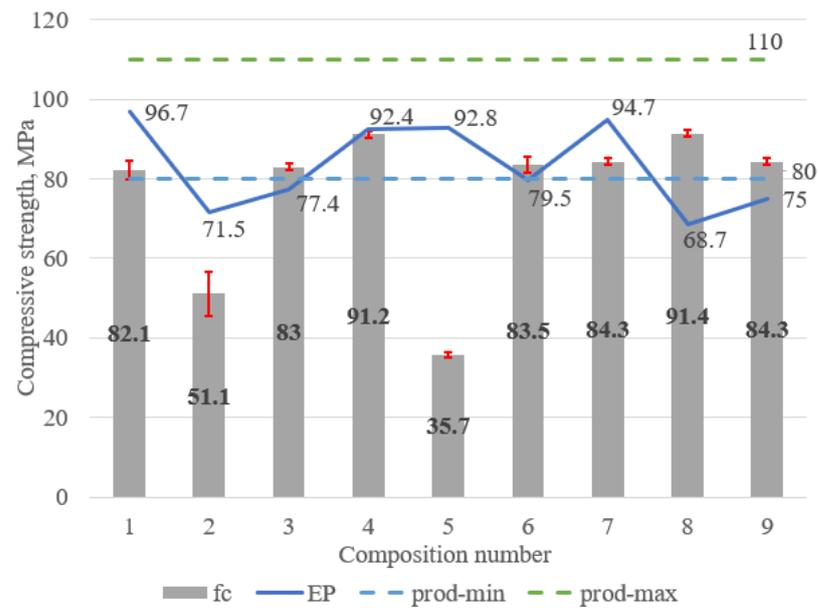
**Figure 9.** Average values of compressive strength with standard deviation presented against the background of the requirements of prefabrication manufacturers and the average results for epoxy mortars.
