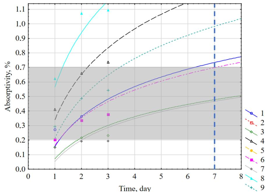
Figure 15. Absorption of mortar samples after the first 7 days of immersion in water compared to the range typical for epoxy mortars (gray rectangle).
