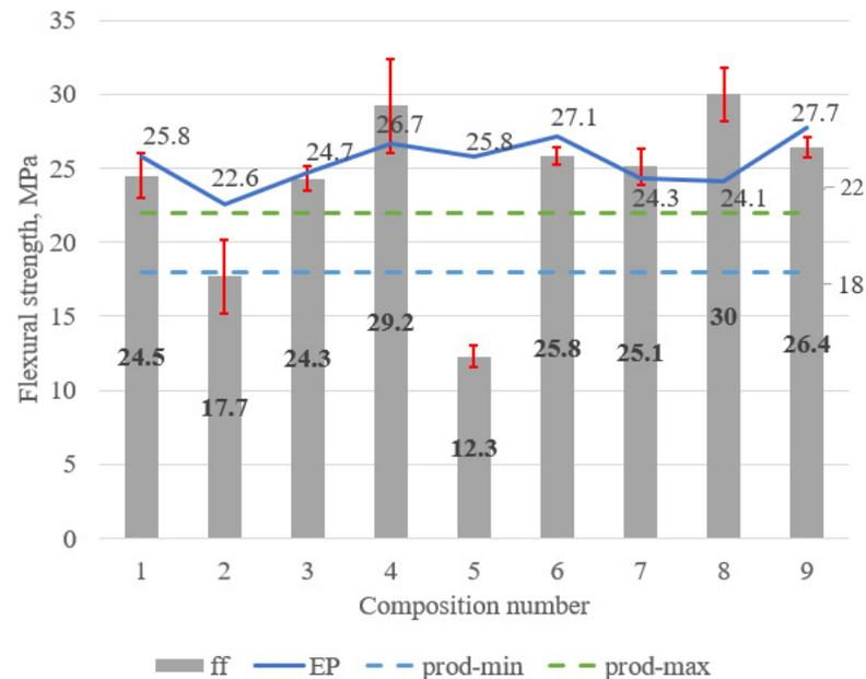
**Figure 8.** Average values of flexural strength with standard deviation presented against the background of the requirements of prefabrication manufacturers and the average results for epoxy mortars.
