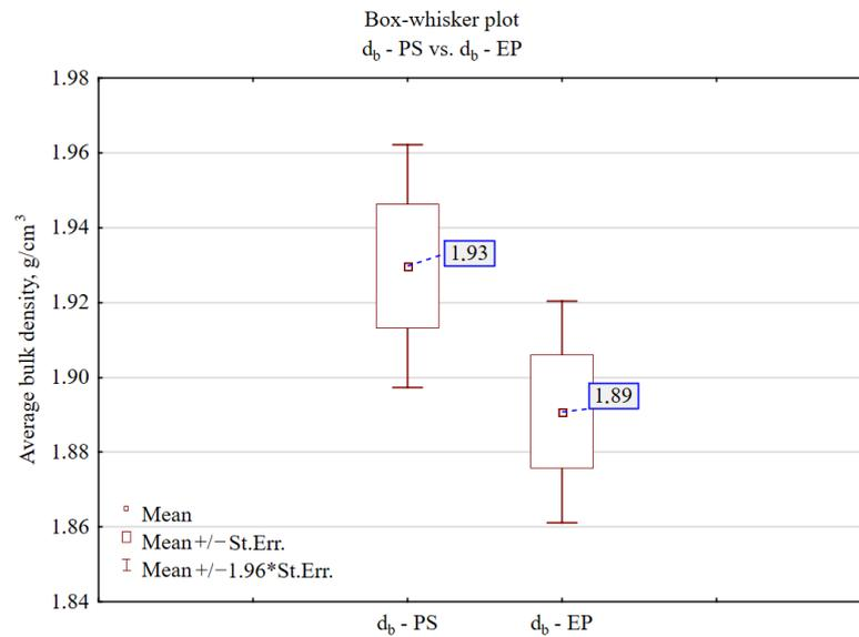
**Figure 13.** Results of the *t*-test presented graphically in the form of box-and-whisker plots for bulk density.
