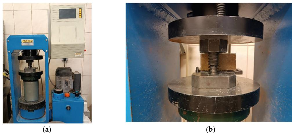
Figure 5. Machine used to test compressive strength: (a) overall view; (b) insert equipped with pressure plates.
