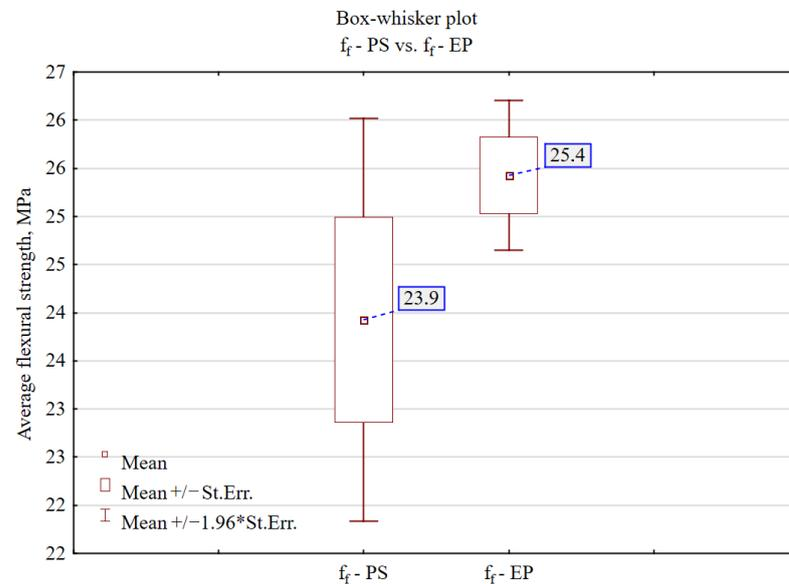
**Figure 11.** Results of the *t*-test presented graphically in the form of box-and-whisker plots for flexural strength.
