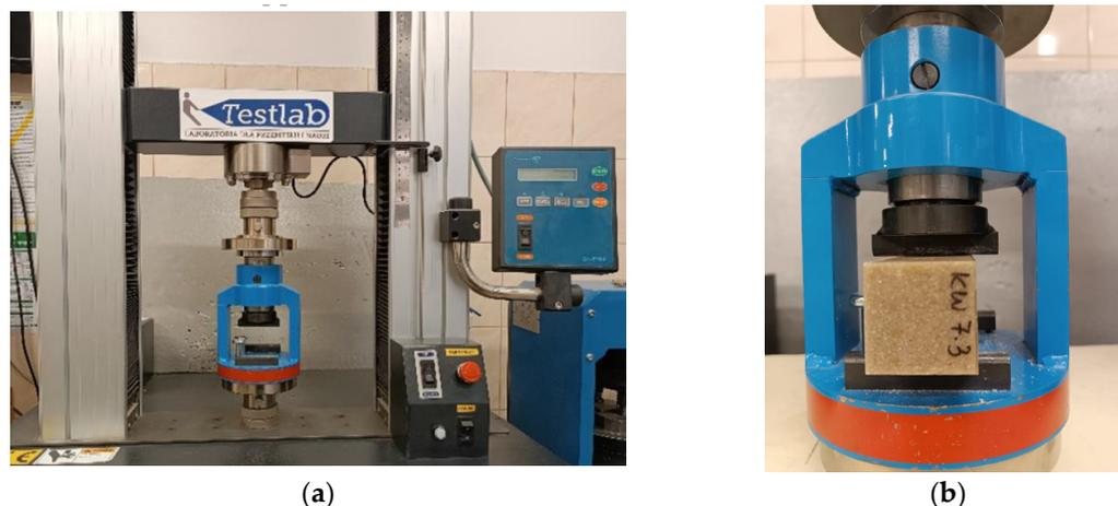
Figure 4. Machine used to test flexural strength: (a) overall view; (b) insert equipped with a flexural system.
