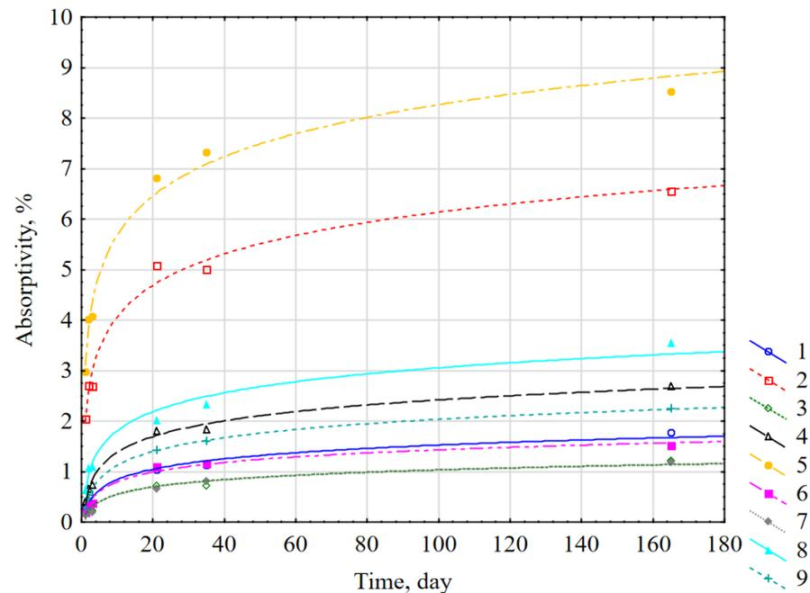
Figure 14. Dependence of the absorbability of mortar samples on the time of immersion in water.
