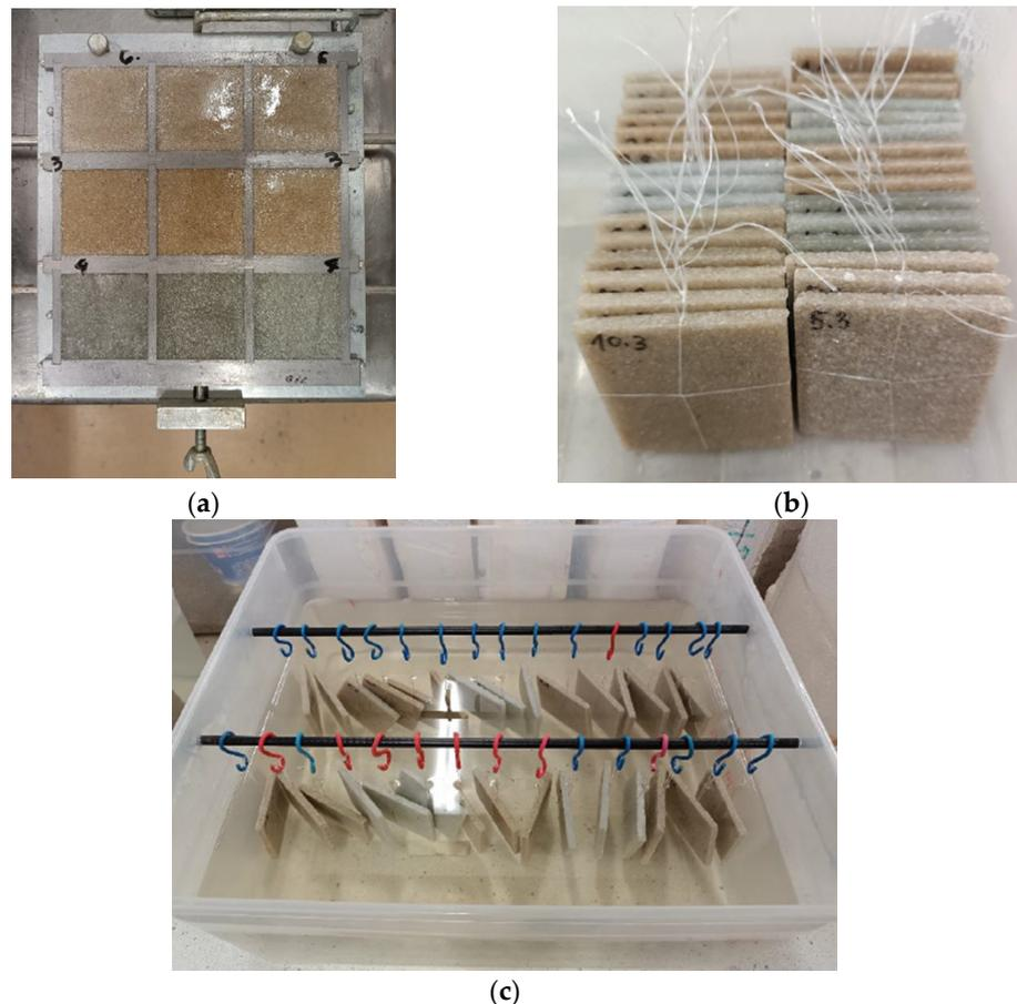
**Figure 6.** Samples intended for absorptivity testing: (a) in metal form; (b) after demolding; (c) after immersion in water.
