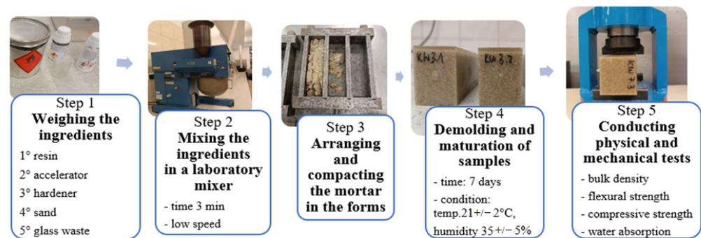
**Figure 2.** Individual stages of preparation of test samples.
