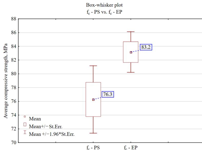
**Figure 12.** Results of the *t*-test presented graphically in the form of box-and-whisker plots for compressive strength.
