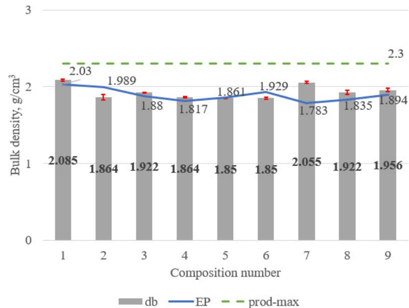
**Figure 10.** Average values of bulk density with standard deviation presented against the background of the requirements of prefabrication manufacturers (prod-max) and the average results for epoxy mortars (EP).
