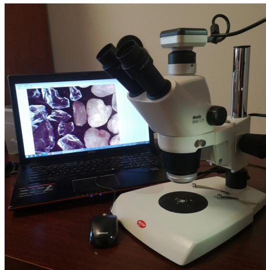
**Figure 3.** The stereoscopic microscope used to take magnified photographs of sand particles and glass waste.
