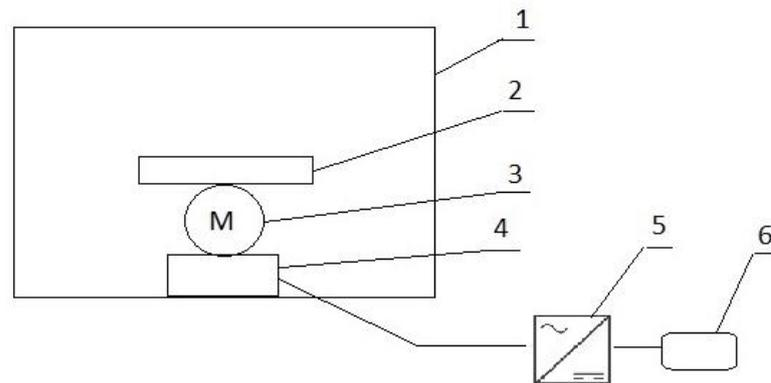
**Figure 3.** Diagram of the vibration simulation stand: 1—stationary vehicle body with adjustable temperature; 2—fruit container; 3—0.09 kW motor, 2800 rpm, 230/400 V, 0.58/0.33 A, IMB3; 4—suspension and vibration isolation (filled with sand); 5—Omron MX2-AB 002-E inverter (SJ200-002NFEF2); 6—computer and software.
