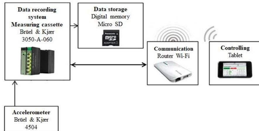
**Figure 1.** Diagram of the vibration measurement stand.
