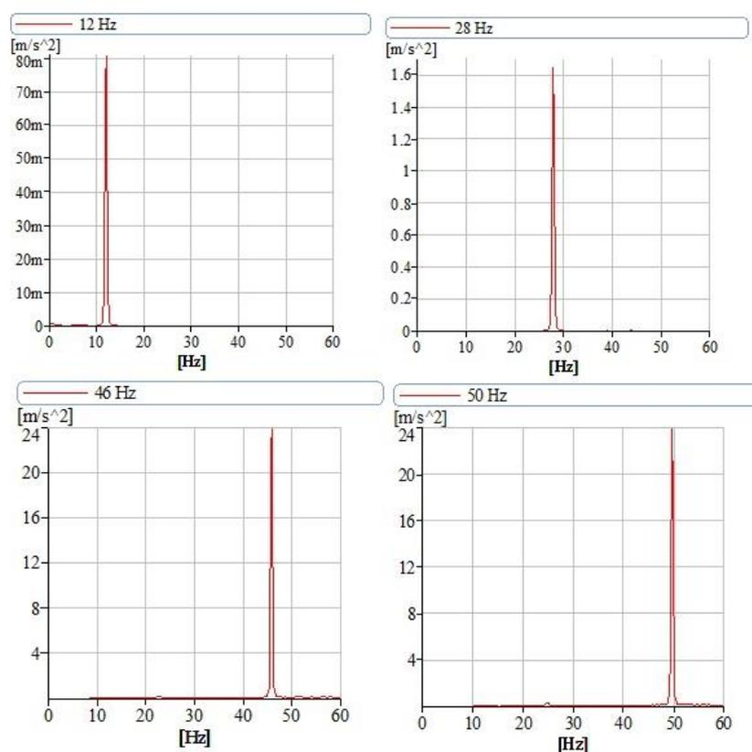
Figure 5. Signal spectra measured on the test stand for different vibration frequencies.
