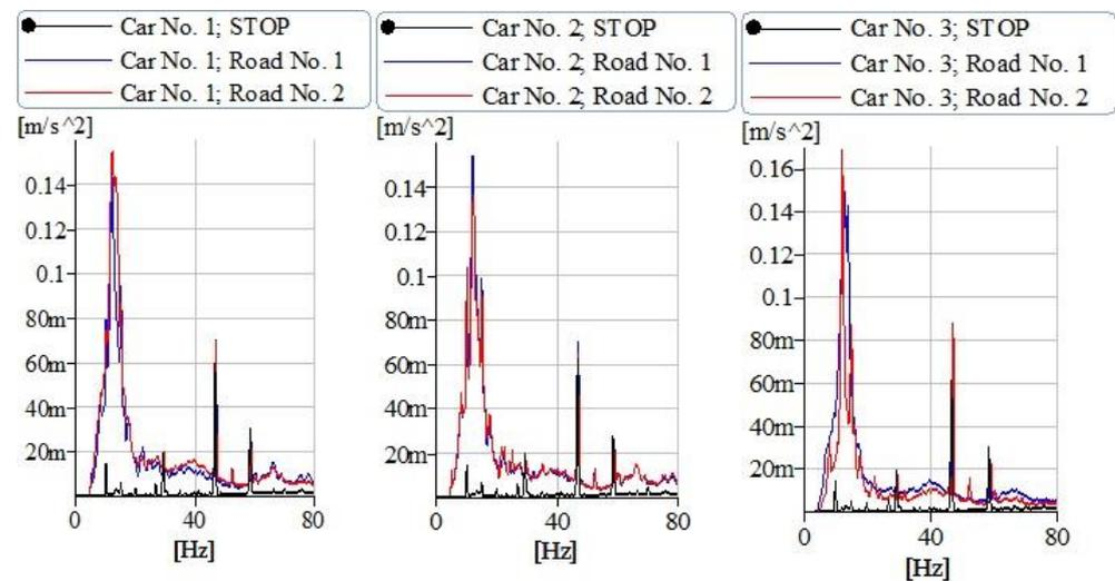
**Figure 2.** Vibration spectrum recorded during the transport under actual traffic conditions.
