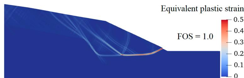
**Figure 19.** Equivalent plastic strain distribution in the high moisture content soil slope subjected to earthquake influence in the limit equilibrium state.
