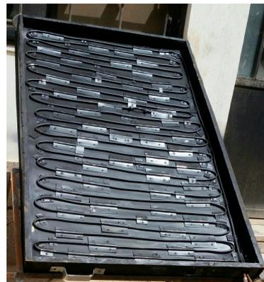
Figure 5. Photograph of flat-plate solar thermal collector (FPSC).
