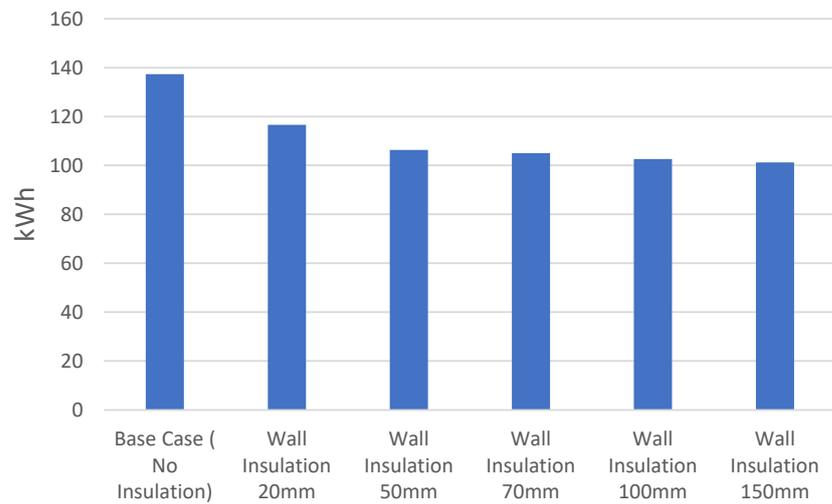
**Figure 12.** Cooling energy usage with insulation added to the external wall.
