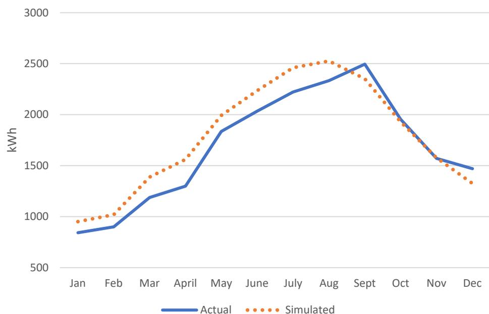
Figure 6. Actual v. modeled monthly electricity use for the base case.
