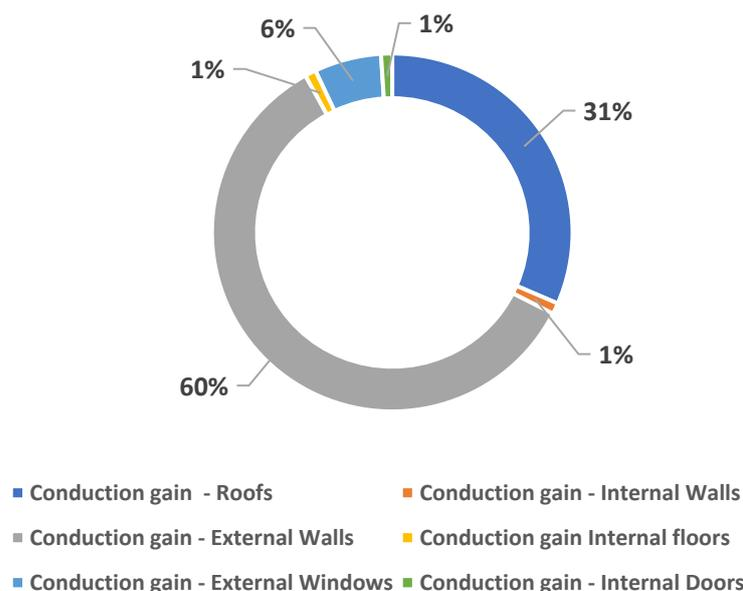
**Figure 10.** Conduction gains breakdown for a bedroom on the first floor.
