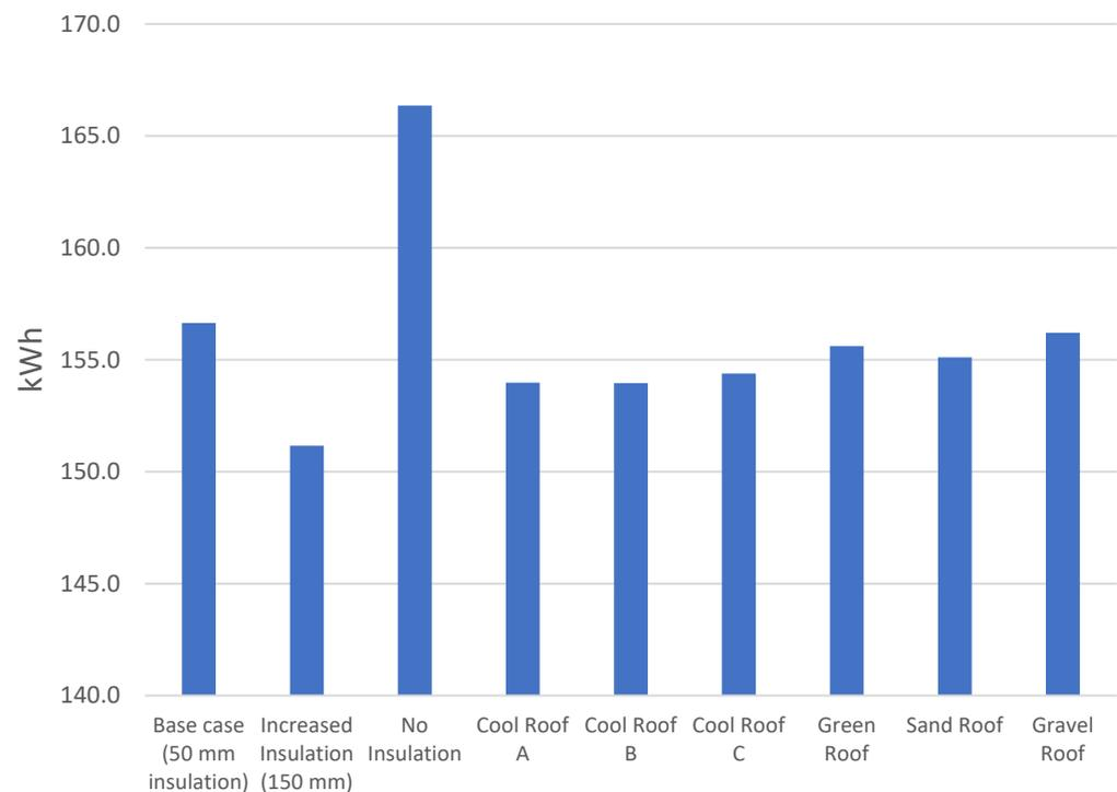
**Figure 8.** Yearly electricity usage for a cooling system for different roof designs.
