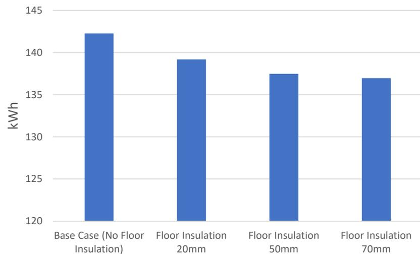
**Figure 13.** Cooling energy usage with insulation added to the ground floor.
