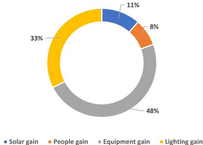
**Figure 9.** Heat gain breakdown analysis for one bedroom adjacent to the roof.
