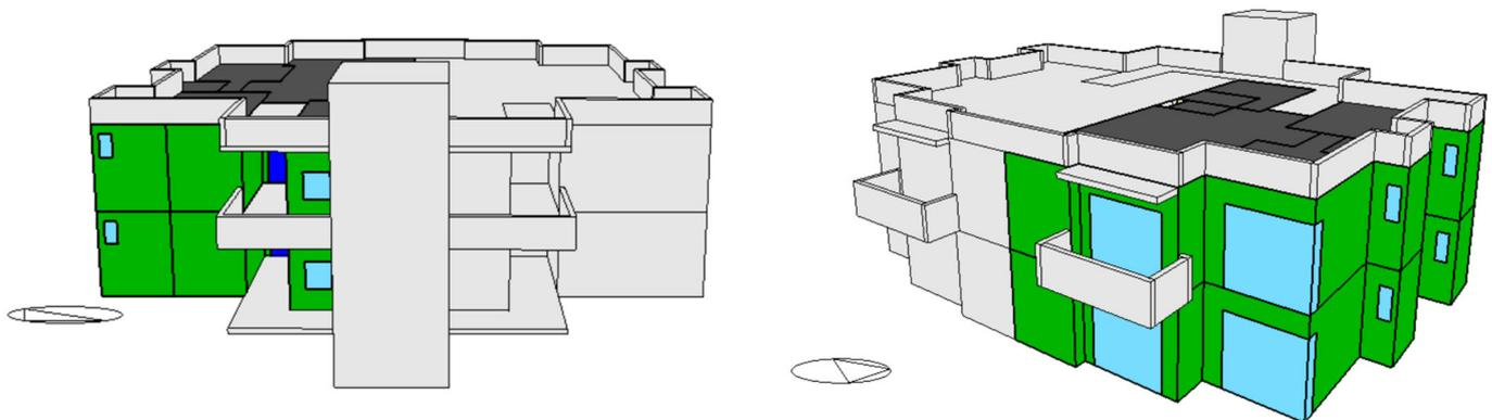
Figure 4. DesignBuilder building model for a typical semi-detached apartment case study. The north arrow on the ground shows the orientation view of the model.
