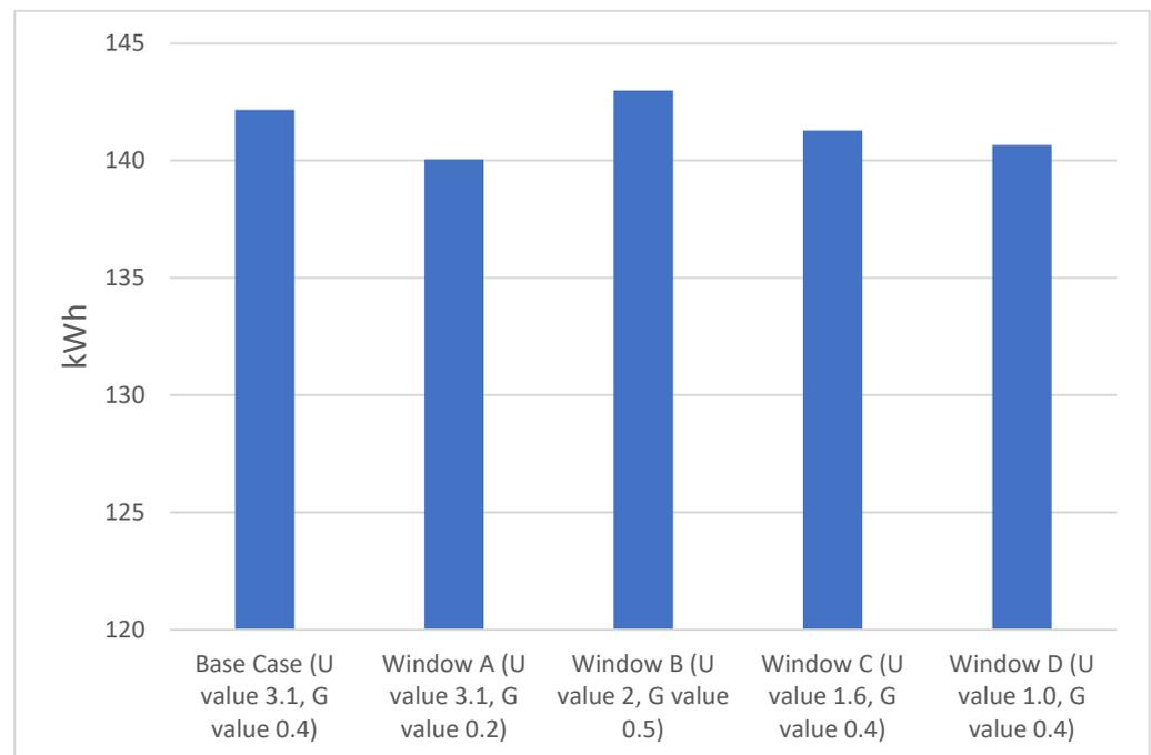
Figure 14. Cooling energy usage for various windows options.
