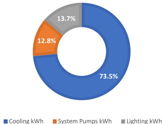
**Figure 7.** Electricity usage in the base case.
