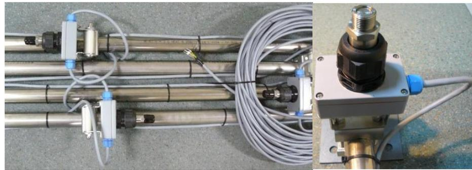
**Figure 2.** Measuring system of bow thruster jet-induced pressure on the quay wall: elements of the measuring system with pressure meters.
