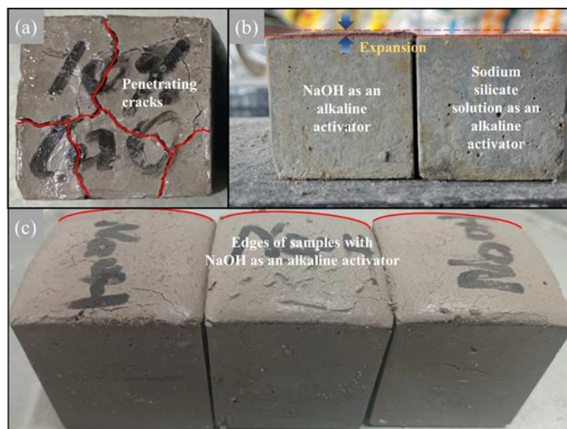
Figure 3. Appearance of AABS samples: (a) excessive amounts of QL, (b) comparison of specimen containing SS with specimen containing QL, (c) excessive amounts of NaOH.
