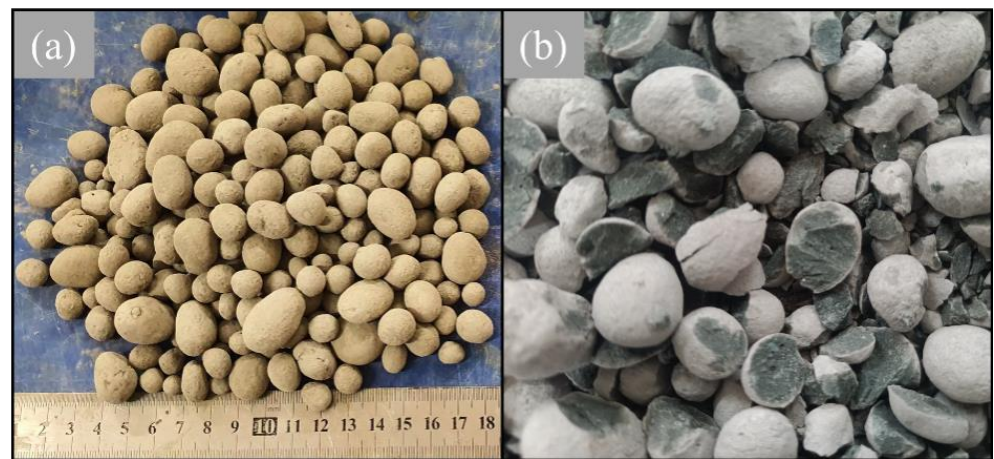
Figure 10. Appearance of SENC: (a) freshly made, (b) after the numerical tube pressure test.
