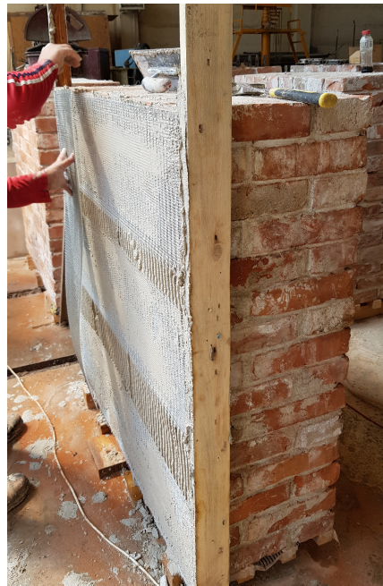
Figure 6. Laboratory testing—one-sided reinforcement of the sample.
