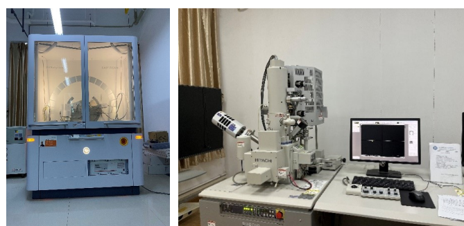
Figure 3. The execution of the XRD and SEM tests.
