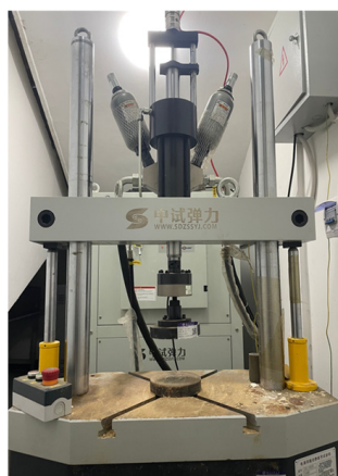
Figure 2. Electro-hydraulic servo dynamic and static fatigue tester. (Note: 中试弹力—ZhongShi Trench).
