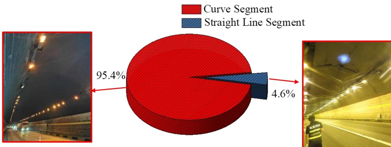
**Figure 9.** The horizontal linear distribution law of traffic accidents.
