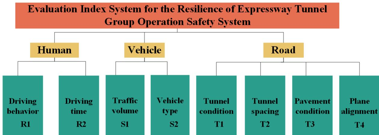
Figure 12. Evaluation index system for resilience of expressway tunnel group operation safety system.
