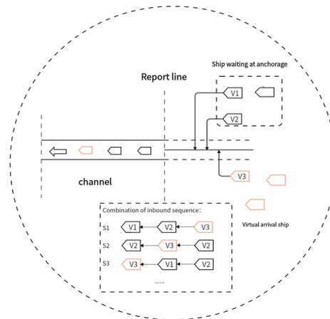
**Figure 1.** Diagram of inbound ship traffic organization through channel (V1, V2 represent ship waiting at anchorage; V3 represents virtual arrival ship; S1–S3 represent the inbound sequence).
