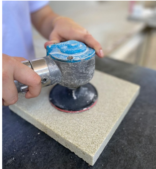
Figure 3. Artificial stone slab produced after honing.
