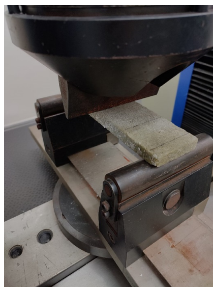
Figure 5. Three-point flexural strength test.
