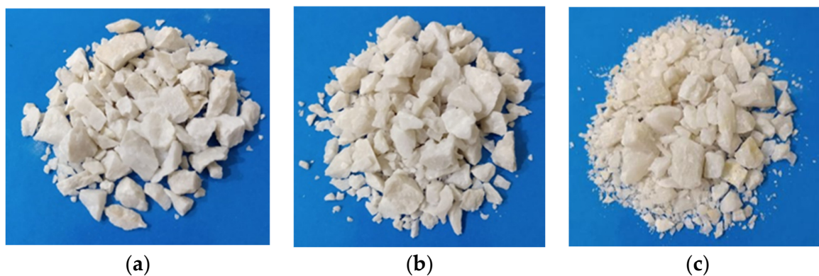
Figure 1. Ornamental stone waste from the quarry: (a) quartzite 1, (b) quartzite 2, and (c) quartzite 3.
