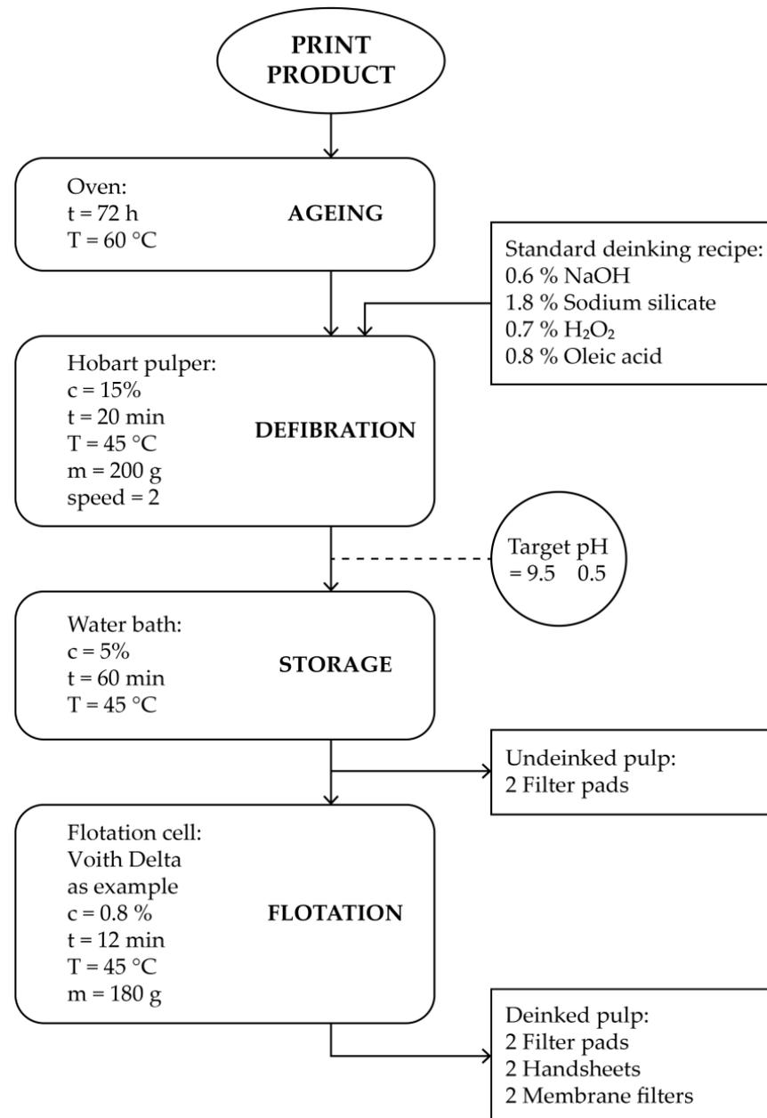
**Figure 2.** Procedure for testing recyclability/deinkability according to INGEDE Method 11 [63].
