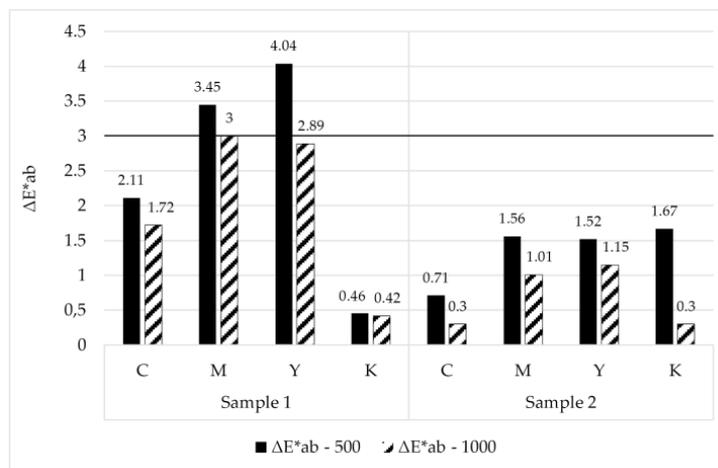
**Figure 5.** Color differences,  $\Delta E^*ab$  of CMYK colors, determined on CMYK prints (Sample 1 and Sample 2) after dry-rubbing treatment with 500 or 1000 rubbing strokes. The line at  $\Delta E^*ab = 3$  indicates an acceptable color change.
