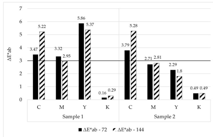
**Figure 3.** Color difference,  $\Delta E^*ab$  of CMYK colors, determined on CMYK prints (Sample 1 and Sample 2) after exposure to light for 72 and 144 h.
