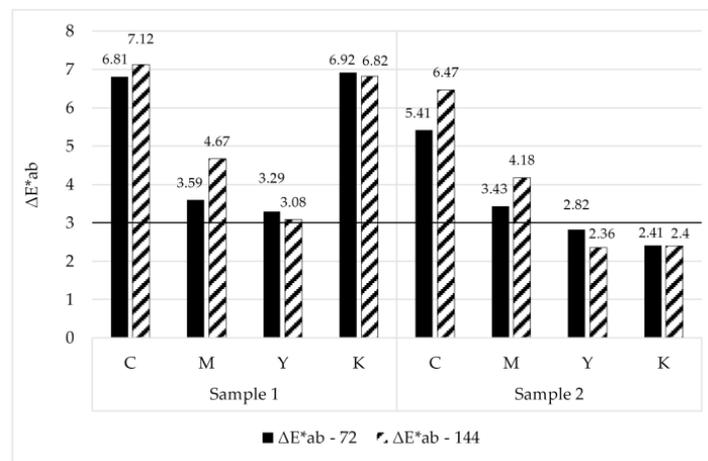
**Figure 4.** Color difference,  $\Delta E^*ab$  of CMYK colors, determined on CMYK prints (Sample 1 and Sample 2) after moist-heat treatment for 72 and 144 h.
