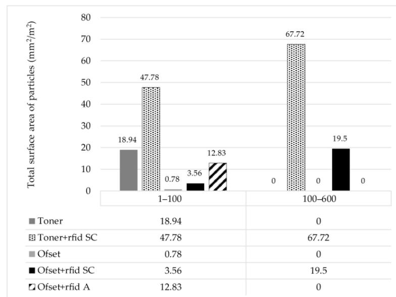
**Figure 7.** The total surface area of particles, i.e., ink residues in deinked samples.
