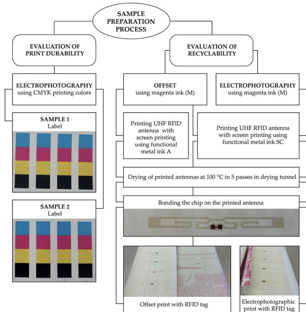
**Figure 1.** Flowchart of sample preparation for evaluation of durability of prints and recyclability of prints.
