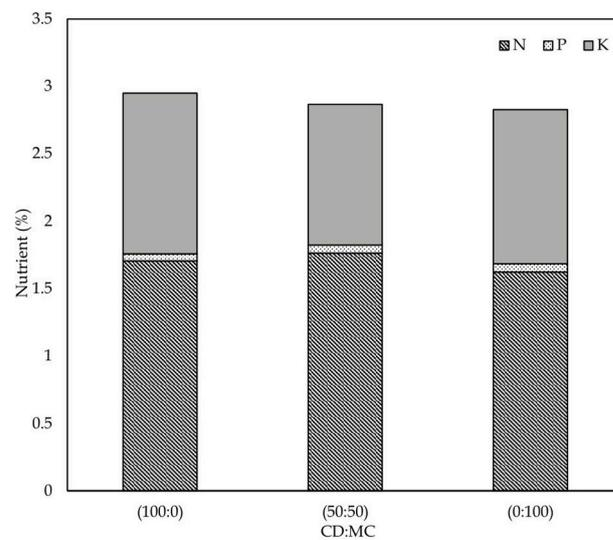
Figure 7. Total nutrient content after digestion at different mixing ratios of CD and MC.
