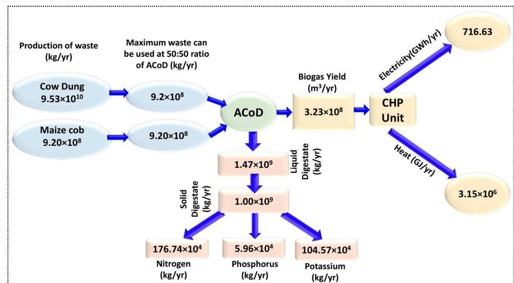
Figure 8. Energy and nutrient production from optimum ratio of CD and MC.
