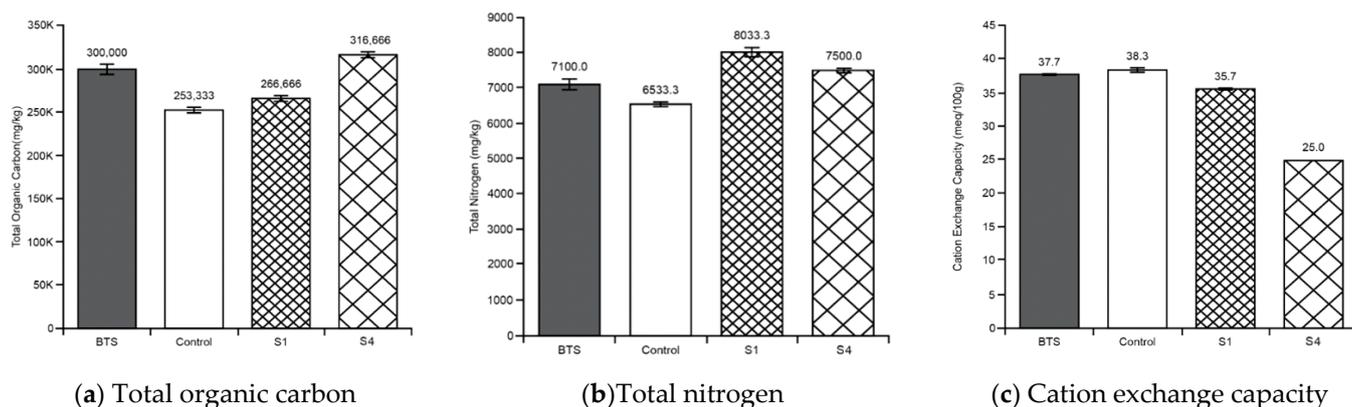
**Figure 11.** Comparison of the physiochemical properties of soil (total organic carbon, total nitrogen and cation exchange capacity) among “Before treatment soil (BTS)”, control soil sample, Stratum 1 (S1) and Stratum 4 (S4).
