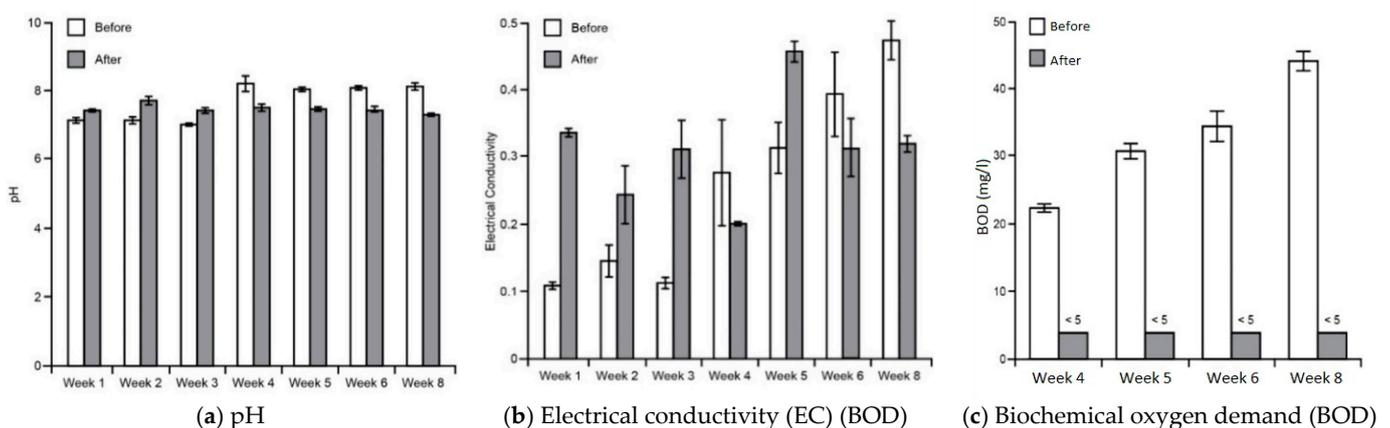
**Figure 8.** Chemical parameters (pH, electrical conductivity and BOD). BODs only measured from week 4–8.
