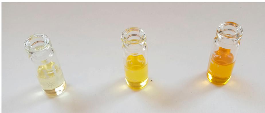
**Figure 4.** Biodiesel samples prepared by TE (left), AE + TE (middle), IEE + TE (right).
