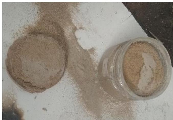
**Figure 6.** Disc sample (left), cut from top of EICP-treated sand specimen (right), used in investigating amounts of calcite precipitation.
