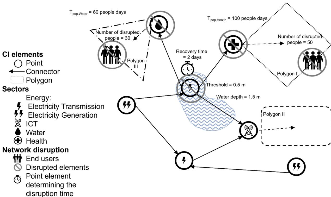
**Figure 2.** Determination of population time  $T_{Pop}$  in a representative small network impacted by a flood [21].
