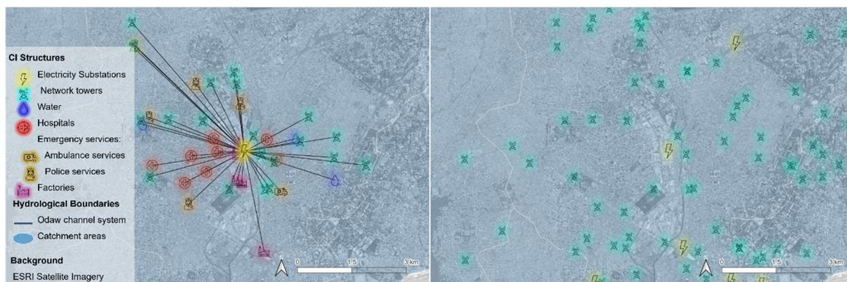
**Figure 10.** Critical infrastructure network elements involved in flood mitigation measures in and around the Odaw river system. (Left) In the centre, an electricity substation is highlighted which is connected to 43 sink elements. (Right) Mobile network towers and electricity substations.
