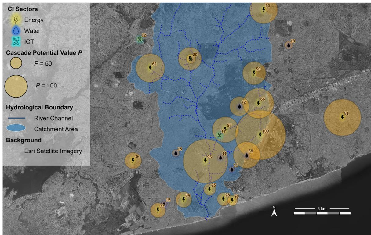
Figure 8. Point elements in the CI network model (V2) of Accra with cascade potential values  $p > 10$  featuring the energy, ICT and water sectors; 1 km radius equals a cascade potential value  $p = 50$  [21].
