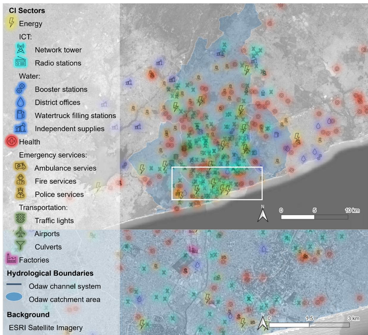
**Figure 5.** Overview of CI network model of Accra, including locations highlighted by CI stakeholders. The highlighted area in the centre of the model shows the proximity of CI network elements to the Odaw channel.
