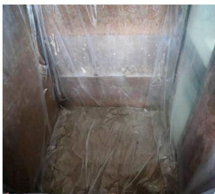
**Figure 4.** Waterproof laying of model box.
