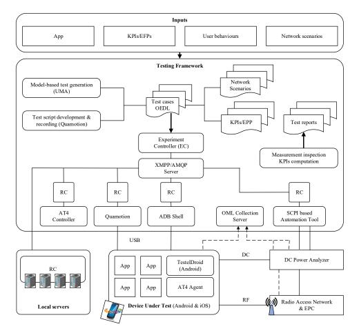
Figure 14. 5G Network Testbed and Benchmarking Scenario.
