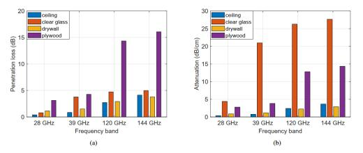
As presented in Figure 15, their result showed a clear increase in attenuation and penetration loss with an increase in frequency.
