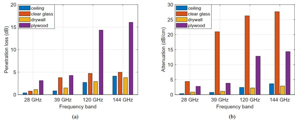
**Figure 15.** A graph showing the results of (a) average penetration loss and (b) average attenuation for ceiling, clear glass, drywall, and plywood at 28, 39, 120, and 144 GHz. The figure was reproduced from a paper [170] titled: Sub-Terahertz and mmWave penetration loss measurements for indoor environments; published in the 2021 IEEE International Conference on Communications Workshops (ICC Workshops).
