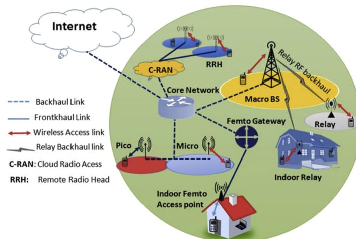
**Figure 8.** Heterogenous Architecture Consisting of Macrocells, Microcells, Picocells, and Femtocells [101].
