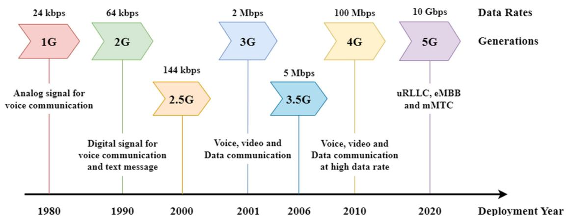
Figure 2. Evolution of cellular communication from 1G to 5G.
