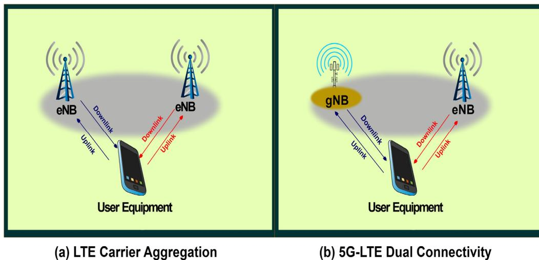
Figure 10. LTE CA and 5G-LTE Dual Connectivity.
