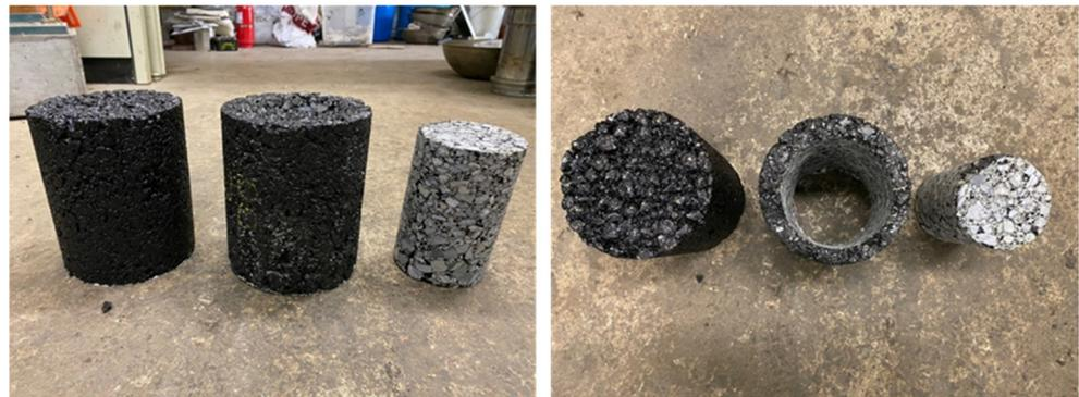
Figure 1. Specimen fabrication using gyratory compactor and cored specimens.
