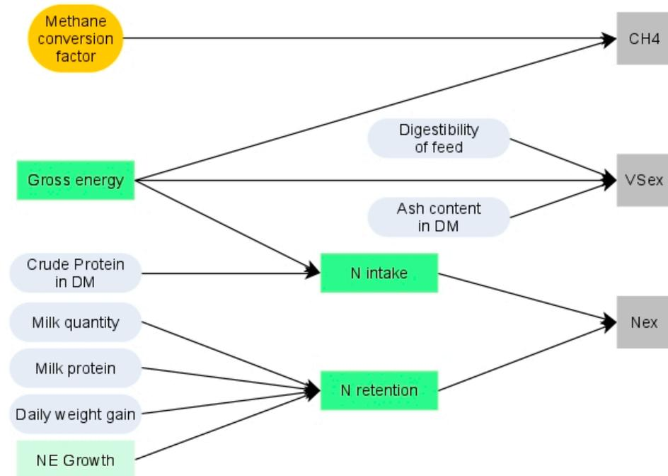
**Figure 2.** Process diagram for the calculation of cattle’s enteric CH<sub>4</sub> emissions, N<sub>ex</sub>, and V<sub>Sex</sub> according to the updated IPCC-2019 method [11]. National average data per livestock category (in blue), the IPCC-2019 conversion factor (in yellow) and the gross energy amount, net energy for growth, and N intake and retention (in green) are used to assess emissions (CH<sub>4</sub>) and excretion (V<sub>Sex</sub>, N<sub>ex</sub>) (in grey).
