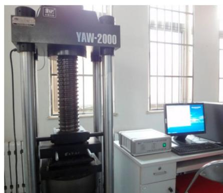
**Figure 7.** The YAW-2000kN-type computer-controlled automatic-pressure testing machine.
