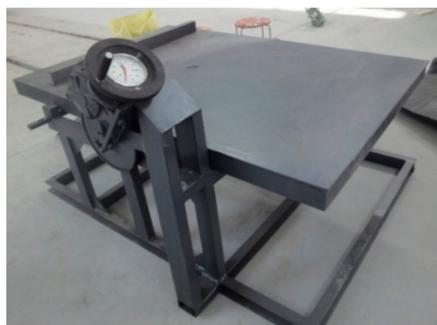
**Figure 3.** The device of the slope sliding experiment.
