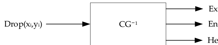
Figure 2. One-dimensional backward cloud generator.
