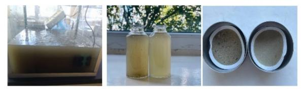
**Figure 4.** Lab experiment: Pre-treatment, samples before and after pre-aeration. TSS content before and after the experiment.
