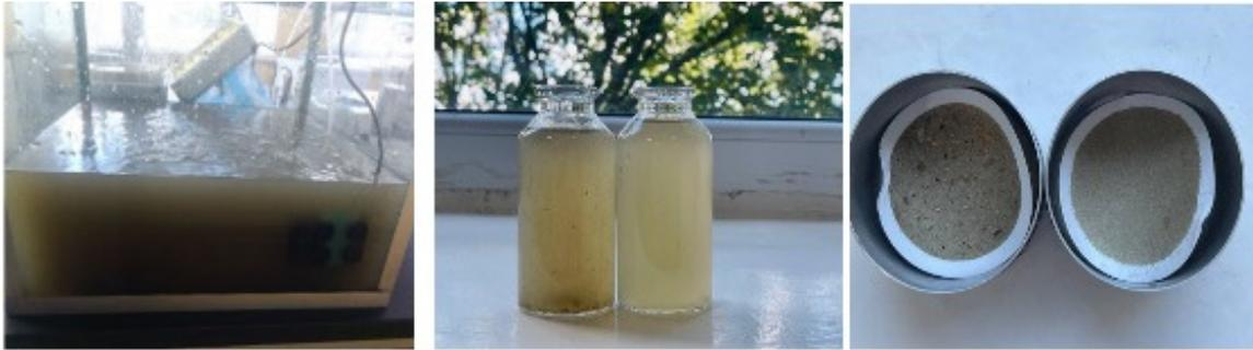
**Figure 4.** Lab experiment: Pre-treatment, samples before and after pre-aeration. TSS content before and after the experiment.
