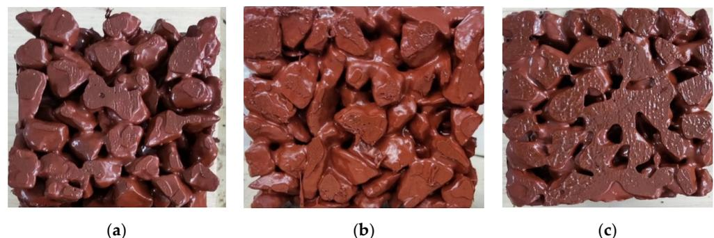
**Figure 9.** Sedimentation diagram of PC samples under different slurry fluidity (a) when the fluidity of the slurry is 105 mm; (b) when the fluidity of the slurry is 115 mm; (c) when the fluidity of the slurry is 130 mm.
