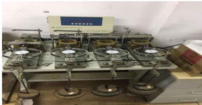
Figure 3. The direct shear test device.
