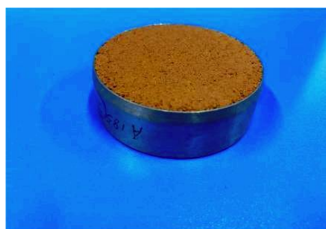
Figure 1. Direct shear test specimens.
