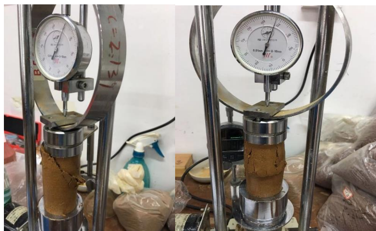
Figure 8. Loading procedure for unconfined compressive strength tests.
