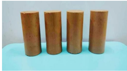
Figure 2. Unconfined compressive strength specimens.
