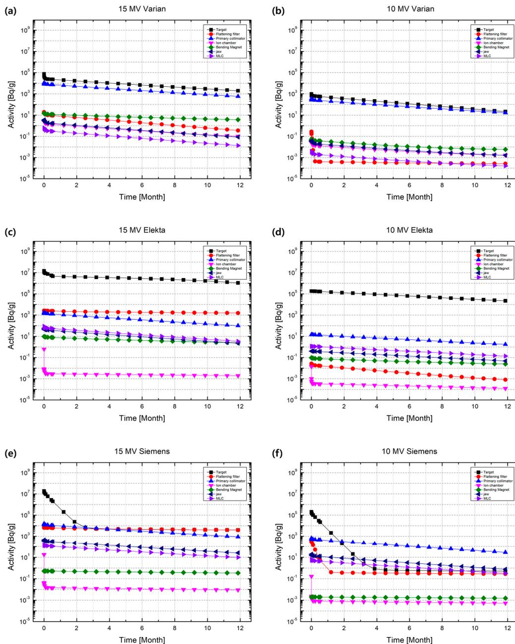
**Figure 3.** Time-dependent changes in the activity levels of the linac major parts obtained by applying a workload of 80 Gy/day at the energy levels of 15 and 10 MV: (a) 15 MV Varian; (b) 10 MV Varian; (c) 15 MV Elekta; (d) 10 MV Elekta; (e) 15 MV Siemens; and (f) 10 MV Siemens.
