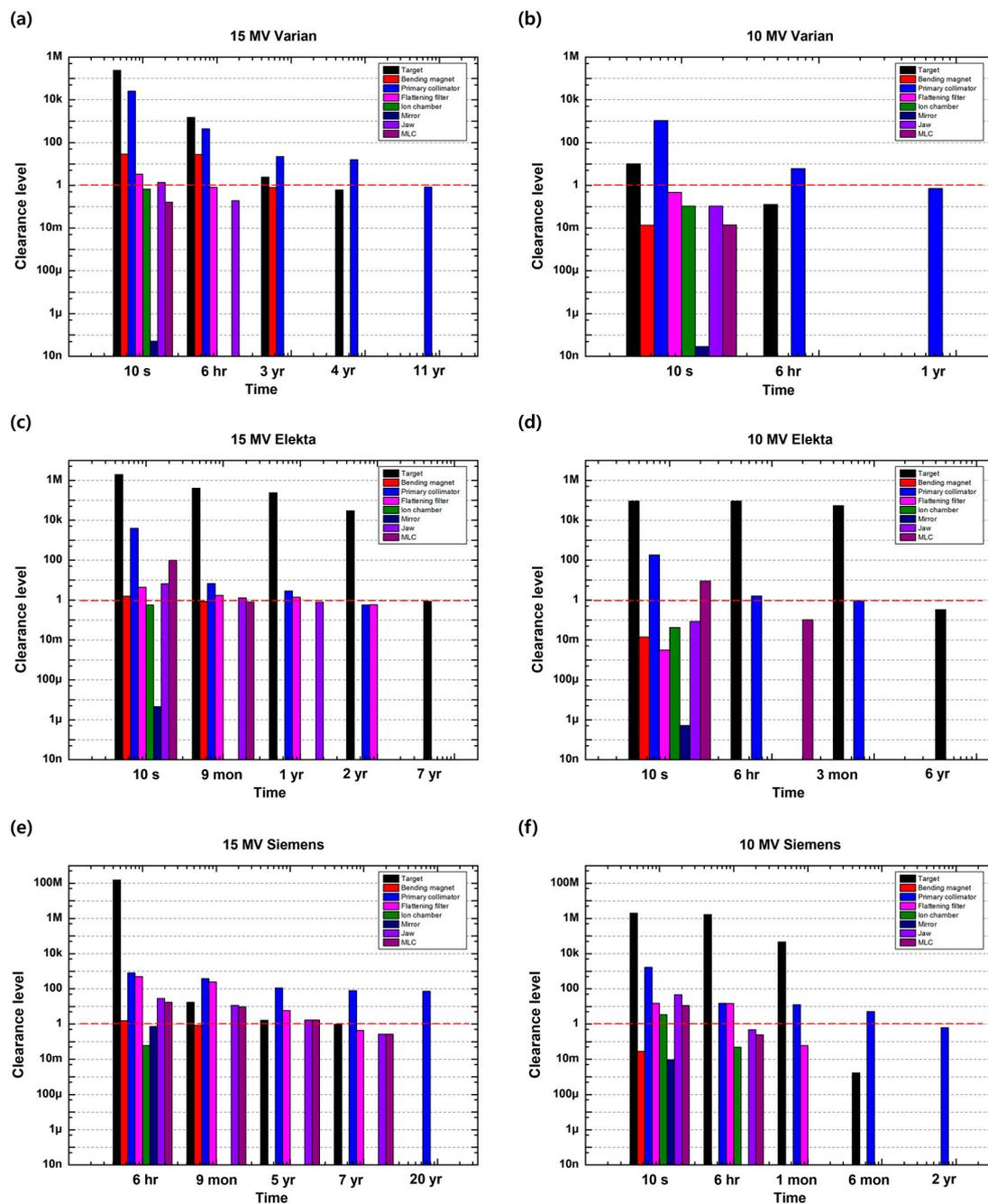
**Figure 4.** Clearance level by part and by equipment (15 MV/10 MV linacs of three manufacturers), applying a workload of 80 Gy/day (dotted red line: reference clearance level of 1; self-disposal is allowed at the activity level below this line): (a) 15 MV Varian; (b) 10 MV Varian; (c) 15 MV Elekta, (d) 10 MV Elekta; (e) 15 MV Siemens; (f) 10 MV Siemens.
