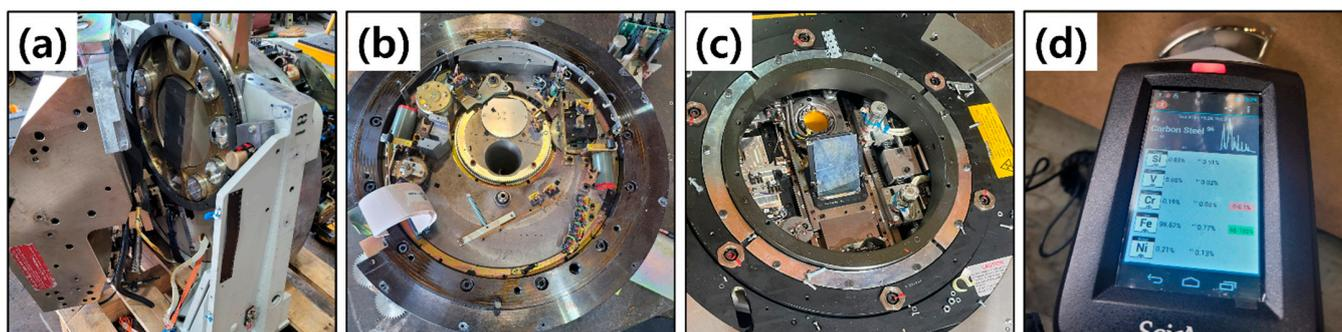
**Figure 1.** Dismantled linac head parts of (a) Clinac iX (Varian); (b) Synergy platform (Elekta); (c) Oncor Expression (Siemens); and (d) LIBS measurement results of the components of their major parts.
