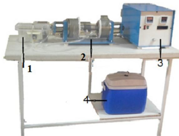
**Figure 1.** Magnetic fuel conditioner device. (1) Fuel tank. (2) The route of fuel rotation. (3) Power supply. (4) Cooling system.
