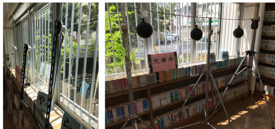
Figure 6. The upper figure shows the arrangement of the measuring instruments. On the left is a cross-sectional view, and on the right is a plan view. The bottom row shows the photos taken during the measurements; the left shows the solar radiation and the right shows the global temperature measurement.
