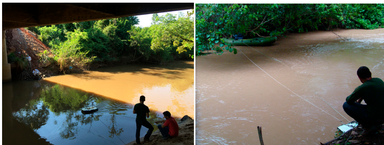
Figure 3. Utilization of the ADCP equipment in obtaining velocities and flows in the studied stretch of the Bois River, using an inflatable boat for displacement from one side to the other of the river.
