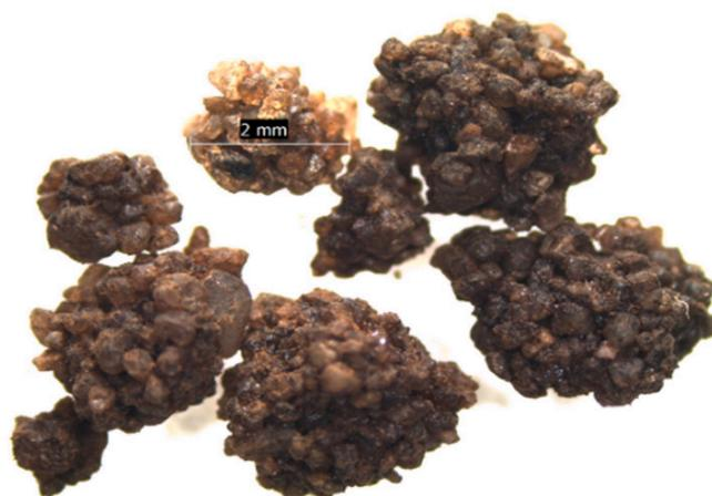
**Figure 3.** Microaggregates of sand particles contaminated by oil hydrocarbons (the image was taken with a LEICA DM750 microscope).
