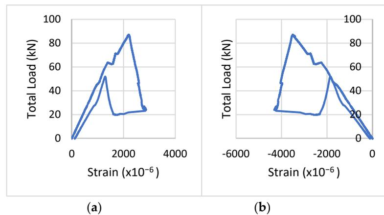
**Figure 7.** Load versus (a) maximum tensile strain and (b) maximum compressive strain at midspan.
