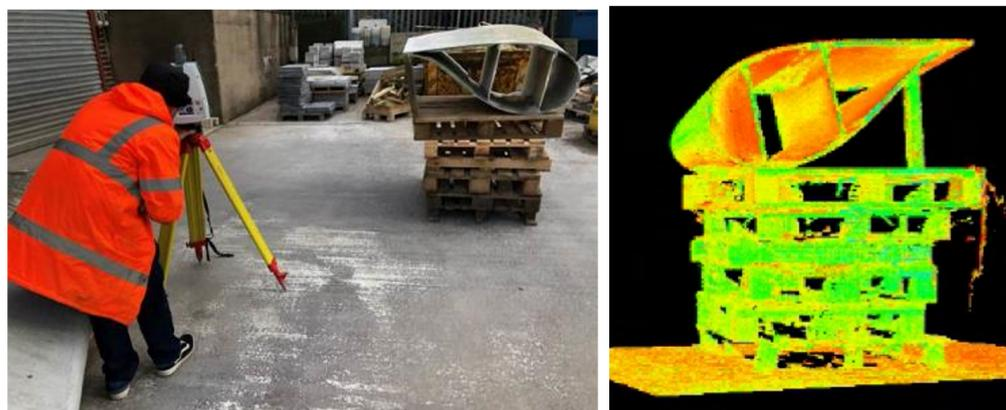
**Figure 2.** LiDAR scanning of one meter long segments.
