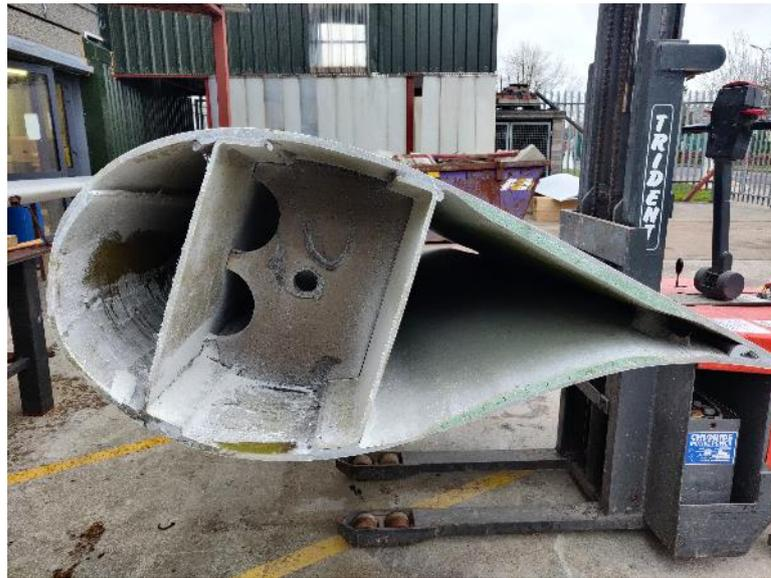
**Figure 3.** Cross-section of the LM 13.4 blade at maximum chord.
