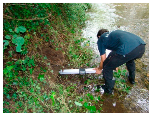
Figure 5. Analysis, by means of a resistograph, of wood deterioration processes in a log crib wall (Artia river, Irún, Guipúzcoa, Spain). Source: Guillermo Tardio.
