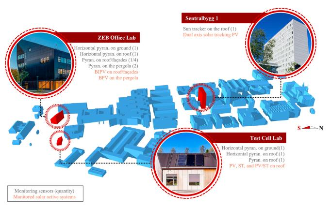
**Figure 2.** Spatial distribution within the NTNU-Solarnet of the monitoring sensors, e.g., horizontally mounted and tilted pyranometers, sun tracker, and the monitored solar active systems, e.g., photovoltaic (PV), building-integrated PV (BIPV), bifacial PV (BPV), solar thermal (ST), hybrid ST/PV, and dual axis solar tracking PV. The experimental facilities of the NTNU-Solarnet that are considered in this study are the Test Cell Lab and the Sentralbygg 1.
