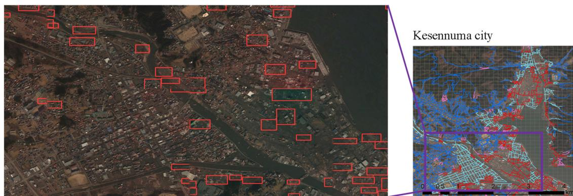
**Figure 13.** Example of the detection results of the traditional method (YOLOv5s).
