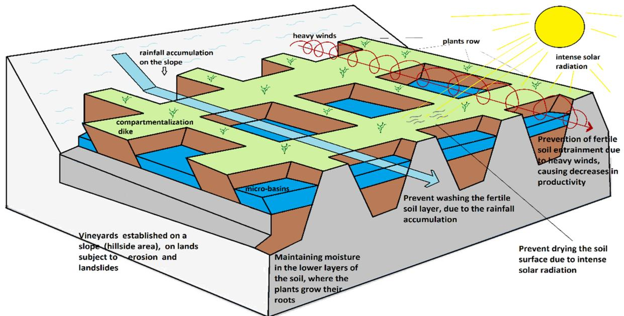
**Figure 1.** Representation of the key advantages resulted from using the furrow diking technology.
