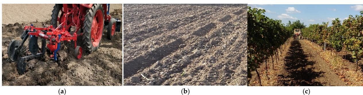
**Figure 5.** Furrow diking equipment operation: (a) operation of the furrow diking equipment attached to an agricultural tractor; (b) micro-basins created with cam-tappet technology; (c) micro-basins construction in the vineyard.
