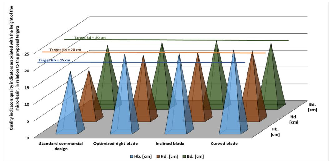
**Figure 12.** Comparative evaluation for three indicators of micro-basin size ( $H_b$ —total height of the dam;  $H_d$ —useful height of the dam;  $B_d$ —width of the dam at the bottom), tested with three new blade shapes.
