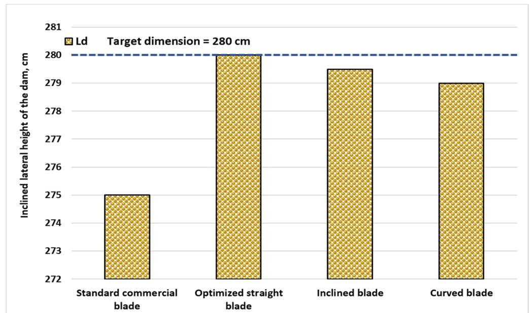
**Figure 14.** Comparative evaluation of the qualitative indicator  $L_d$  (length between two dams), for the proposed constructive rotor blades.
