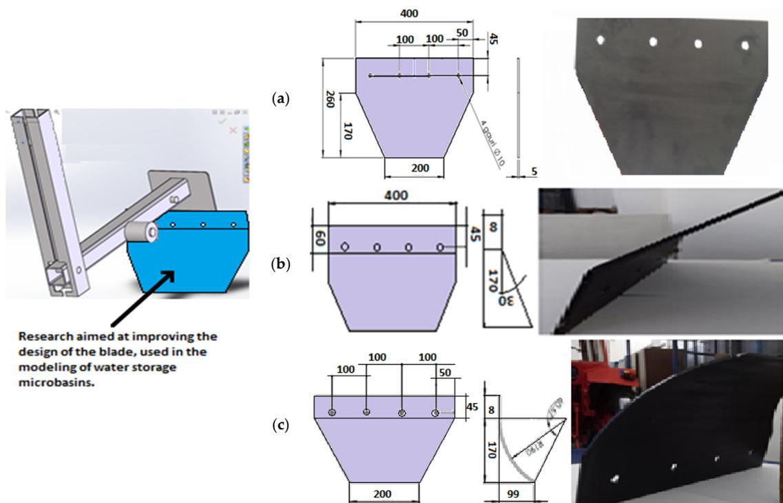
**Figure 8.** Design of three new optimized blades for the furrow compartmentation equipped: (a) straight blade; (b) inclined blade; (c) curved blade.
