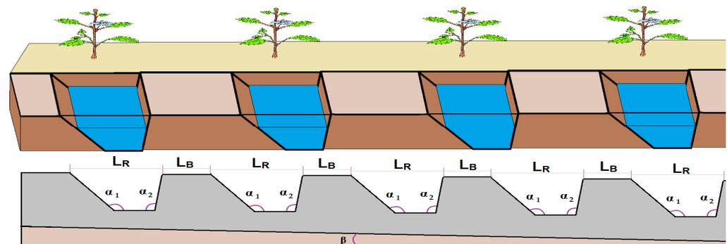
**Figure 16.** Principles regarding the customization of the micro-basins using the cam-tappet system.
