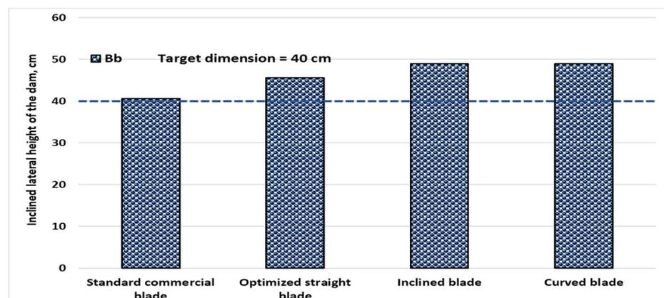
**Figure 13.** Comparative evaluation of the qualitative indicator  $B_b$  (width height of the dam at the top), for the proposed constructive rotor blades.
