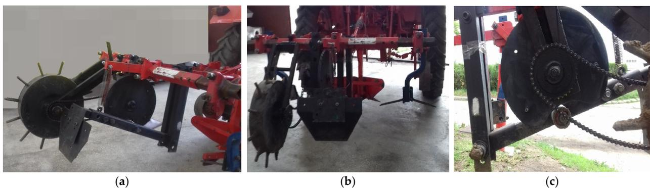
**Figure 4.** The furrow diking system mounted on an agricultural tractor: (a) side view; (b) back view; (c) cam-tappet mechanism and the driving chain.
