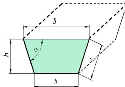
**Figure 7.** Determining the mathematics of micro-basin cross section characteristics.
