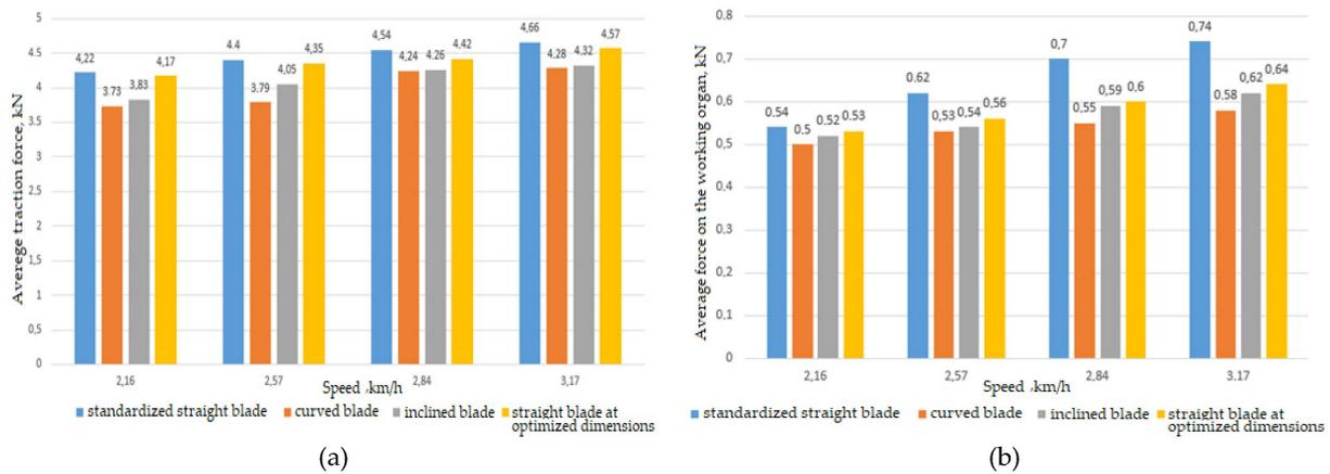
**Figure 11.** Study of the forces employed in the furrow diking system operation: (a) Variation of the average traction force as a function of speed; (b) Variation of the average force on the working organ as a function of speed.
