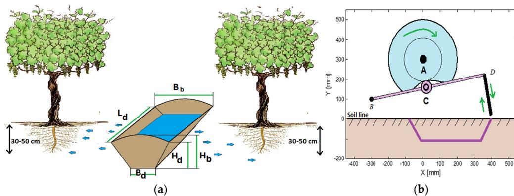
**Figure 6.** Furrow diking technology assessment: (a) Establishing the main gauge indicators: depth of watering ditch ( $H_d$ ), the width at the bottom ( $B_d$ ); the upper width of the ditch ( $B_b$ ), dam height ( $H_b$ ), the distance between dams ( $L_d$ ); (b) Principle of maneuvering the hoe using the cam-tappet mechanism.
