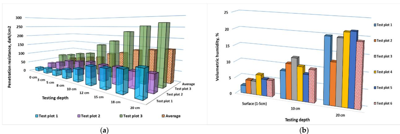
**Figure 9.** Evaluation of soil penetration resistance (a) and volumetric soil moisture (b) as a function of soil-depth.
