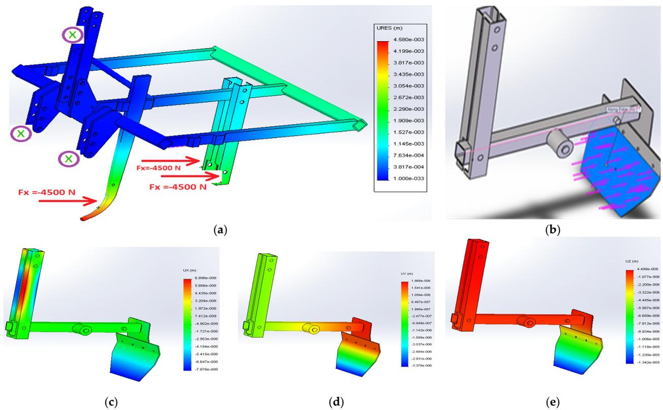
**Figure 10.** Analysis of the stresses in the frame and the hoe—supporting arm subassembly: (a) The structural model of the supporting frame with the distribution of the relative displacements; (b) The structural model of the tillage hoe; Distributions of the relative displacement field (deformation) of the hoe along the X axis (c), along the y axis (d) and along the Z axis (e).
