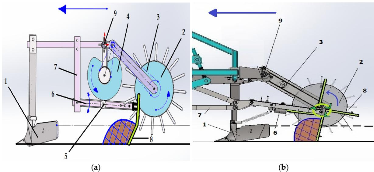
**Figure 15.** The operating principles of two systems used for opening and partitioning water furrows: (a) Equipment operating using the cam-tappet principle; (b) Equipment operating on the mobile rotor principle. Main components of the two furrow diking systems: 1—arrow knife for hoeing, 2—spur wheel for driving the compartmenting mechanism, 3—chain drive, 4—cam, 5—tappet, 6—supporting frame, 7—arm support, 8—compartmentation blades, 9—camshaft axle.
