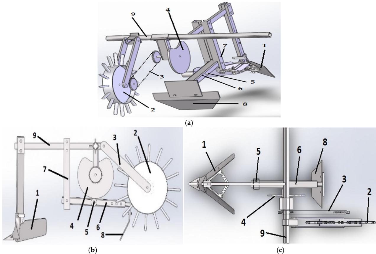
**Figure 3.** Description of the proposed furrow diking equipment main components, operating using the cam-tappet mechanism: (a) panoramic view; (b) side view (c) top view. Equipment simplified technical scheme consisting of: 1—bushing plough, 2—spur wheel, 3—chain drive, 4—camshaft, 5—tappet, 6—supporting arm, 7—supporting bar, 8—soil collection blade, 9—frame supporting working organs.
