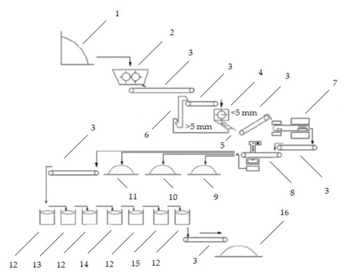
**Figure 4.** Diagram of a technological line for the utilization of photovoltaic panels: (1—photovoltaic cell laminate storage, 2—two-shaft shredder, 3—belt conveyor, 4—hammer crusher, 5—screen, 6—bucket conveyor, 7—furnace, 8—multisensor separator, 9—copper storage, 10—metal storage, 11—glass warehouse, 12—rinsing, 13—alkaline etching, 14—acid etching, 15—etching with a three-component mixture, 16—silicon store). Source: Own study.
