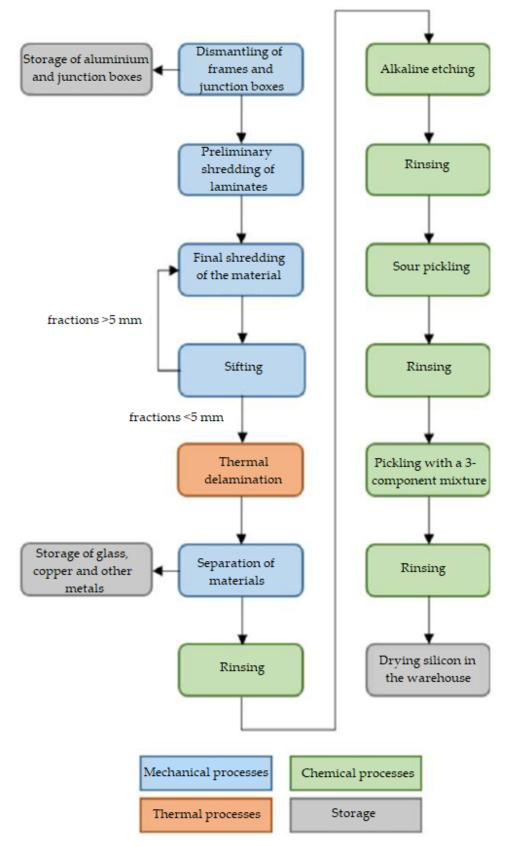
**Figure 2.** Block diagram of the process of recycling photovoltaic panels, taking into account the type of process. Source: Own study.
