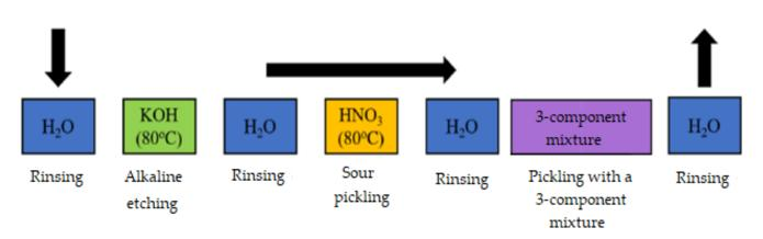
Figure 3. Stages of the chemical process. Source: Own study.
