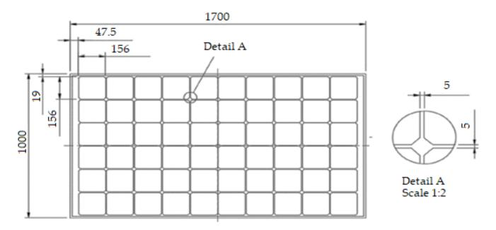
Figure 1. Sketch of a standard PV panel. Source: Own study.
