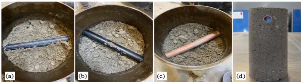
**Figure 2.** (a–c) RL-CBR sample preparation with HDPE, PE, and copper pipes. (d) Prepared RLT sample with a copper pipe.
